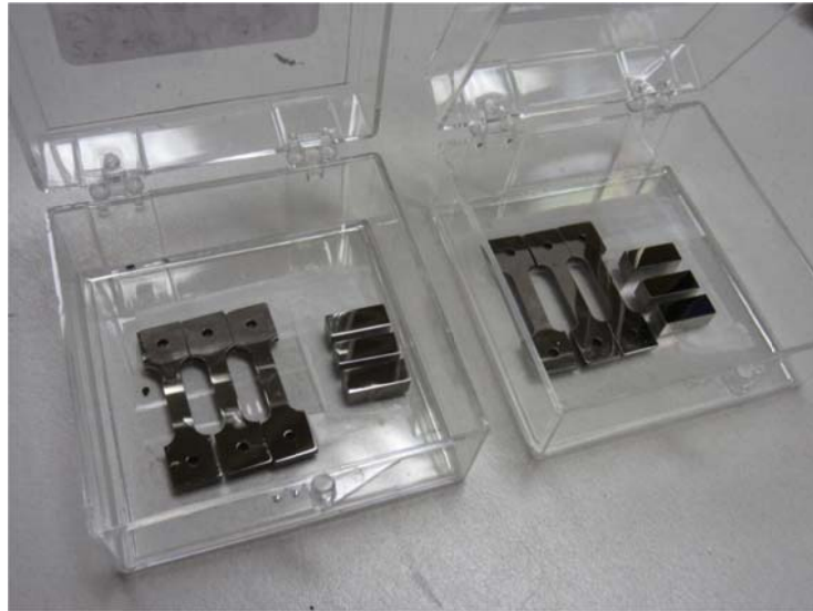
Figure 4.18. Preparation of the TiAl samples. The samples are polished with SiC paper (from P800 up to P4000), and successively etched.
