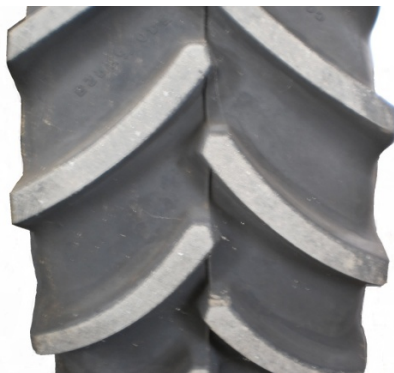
Figure 3.50: tread pattern of the tyre modeled for the simulations performed considering the interaction with a multi-body model of the whole tractor
