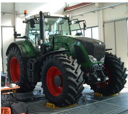
Figure 3.44: tested vehicle on the four-post test rig.
