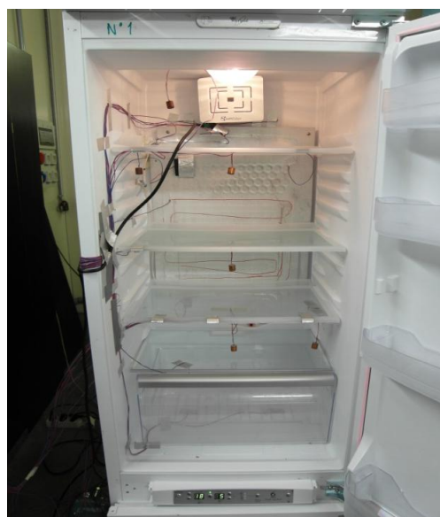
Figure 2.3 Visible roll-bond evaporator in SDE circuit prototype refrigerator-freezer
