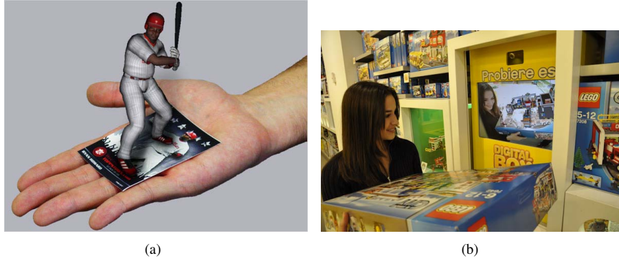
Figure 7.1: Examples of image-based natural features tracking for AR. On the left, the tracking system relies on a picture card to perform the augmentation. On the right, a marketing AR application from LEGO®; the system recognizes the box and it superimpose the 3D model of the construction on top of it.
