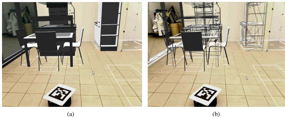
Figure 9.6: Object highlighting. If the user does not select any particular object, all the virtual pieces of furniture are correctly visible (a). When an object is selected (b), all the others are visualized in wireframe mode.
