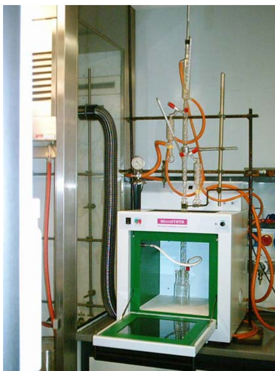
Figure 2.6 - ETHOS 1600 Microwave Reactor from Milestone (Bg) used in the synthesis of DGDC. (35 x 35 x 35 cm); max power 1000 Watt - 2 industrial magnetron (800 W power) cooled by high flow fans MW supplied in a mixing chamber and distributed by a metallic Diffuser located on back wall.
