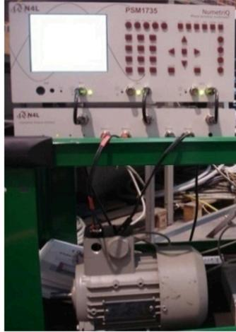
FIGURE 2.13 MEASUREMENT WITH LRC BRIDGE ON 1.1KW AC INDUCTION MOTOR.
