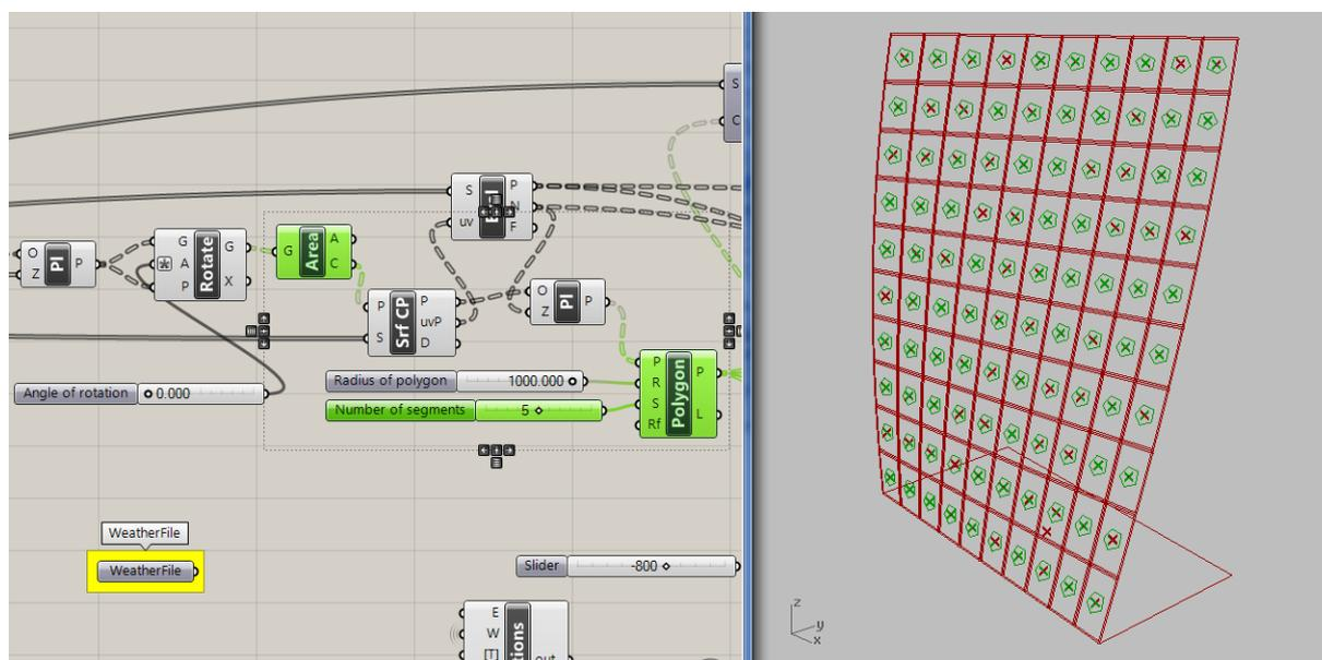
Figure 65. *Grasshopper* definition (on the left) with the profile of the panels visualized in *Rhinoceros* work environment (on the right)
