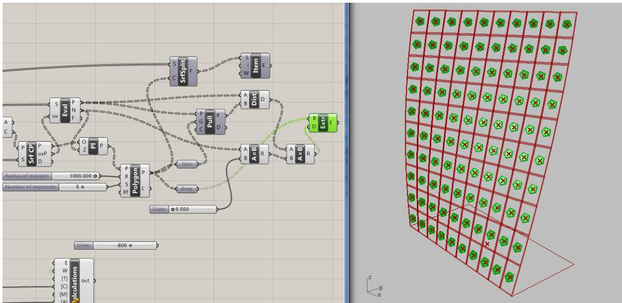
Figure 66. *Grasshopper* definition (on the left) with the extrusion of the panels visualized in *Rhinoceros* work environment (on the right)
