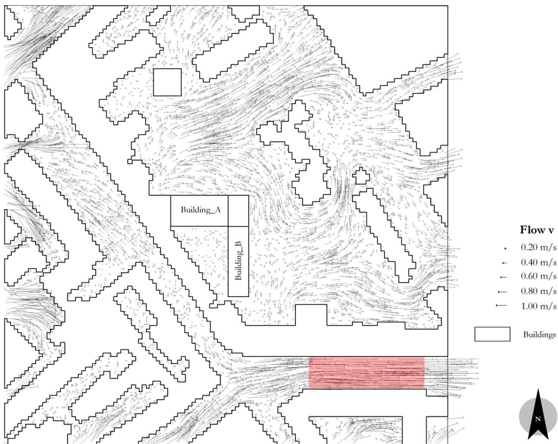
Figure 102. Current scenario: horizontal section at ground level, wind speed vectors at 3:00 p.m. on the 16th of June
