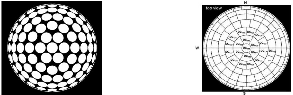
Figure 8. Sky division schemes: (on the left) according to Tregenza: 145 sky segments with a cone opening angle of 10.15°, with 68% of the celestial hemisphere covered by sky segments; (on the right) continuous division, as used by *Daysim*
