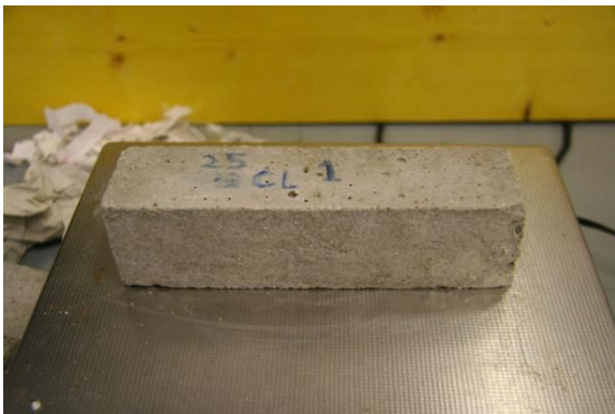
Fig 156 25% Lime Cement Sample 1 Right after 93 Cycles, Left New sample
