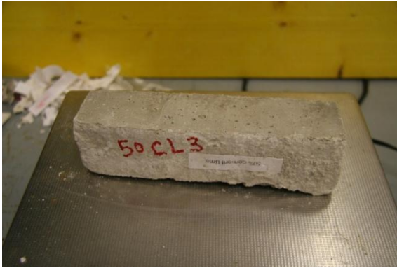
Fig 163 50% Lime Cement Sample 3 Right after 93 Cycles, Left New sample
