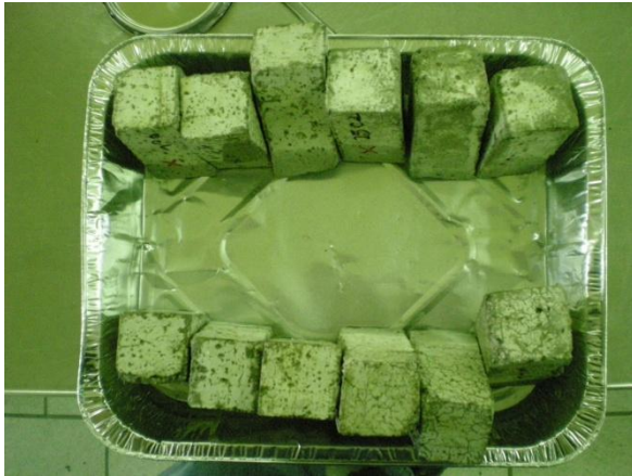
Fig 99 Samples for Water Absorption Test.
