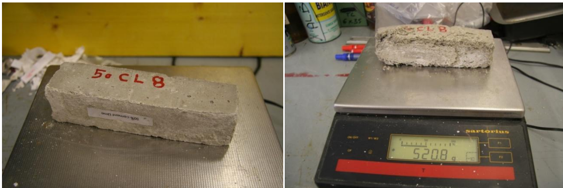
Fig 123 50% Cement Lime Sample 8 Right after 50 Cycles, Left New sample
