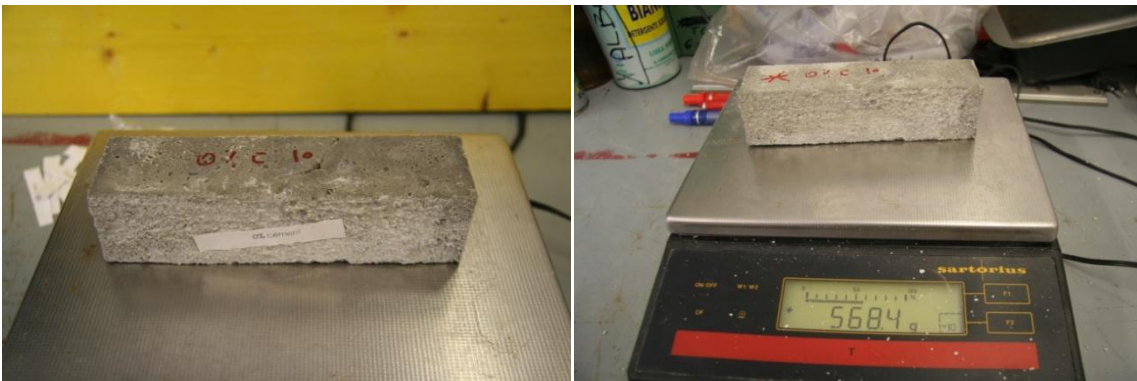
Fig 135 0% Cement Sample 10 Right after 50 Cycles, Left New sample
