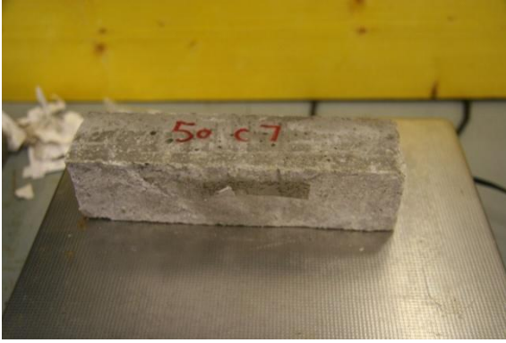
Fig 142 50% Cement Sample 7 Right after 50 Cycles, Left New sample
