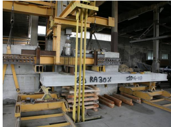
Fig 16 bending test on Beam Made of recycled aggregate concrete [49]
