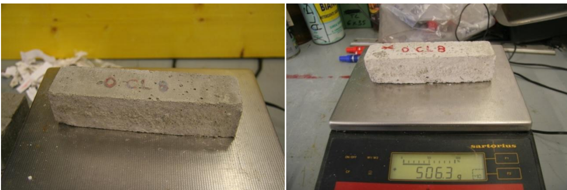
Fig 113 0% Cement Lime Sample 8 Right after 50 Cycles, New sample
