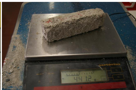
Fig 166 100% Lime Cement Sample 1 Right after 93 Cycles, Left New sample
