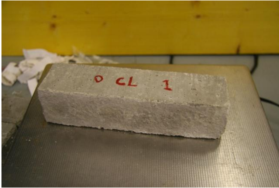
Fig 151 0% Lime Cement Sample 1 after Right 93 Cycles, Left New sample
