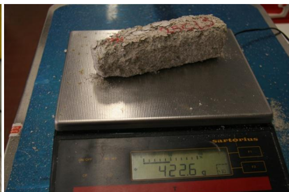
Fig 158 25% Lime Cement Sample 3 Right after 93 Cycles, Left New sample
