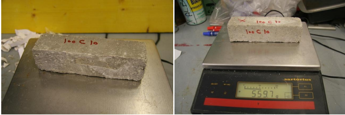
Fig 150 100% Cement Sample 10 Right after 50 Cycles, Left New sample
