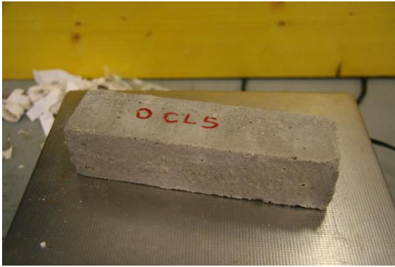
Fig 155 0% Lime Cement Sample 5 Right after 93 Cycles, Left New sample
