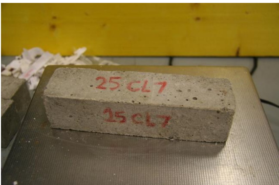
Fig 117 25% Cement Lime Sample 7 Right after 50 Cycles, New sample
