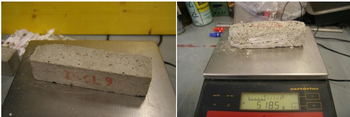
Fig 119 25% Cement Lime Sample 9 Right after 50 Cycles, New sample
