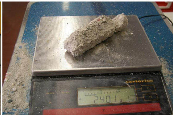
Fig 168 100% Lime Cement Sample 3 Right after 93 Cycles, Left New sample
