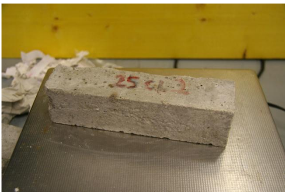
Fig 157 25% Lime Cement Sample 2 Right after 93 Cycles, Left New sample
