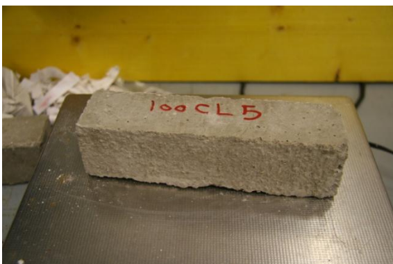
Fig 170 100% Lime Cement Sample 5 Right after 93 Cycles, Left New sample
