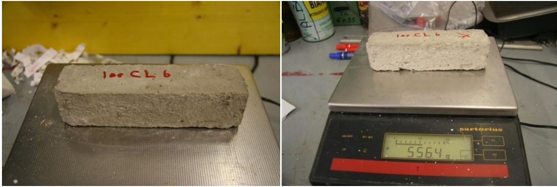
Fig 126 100% Cement Lime Sample 6 Right after 50 Cycles, Left New sample
