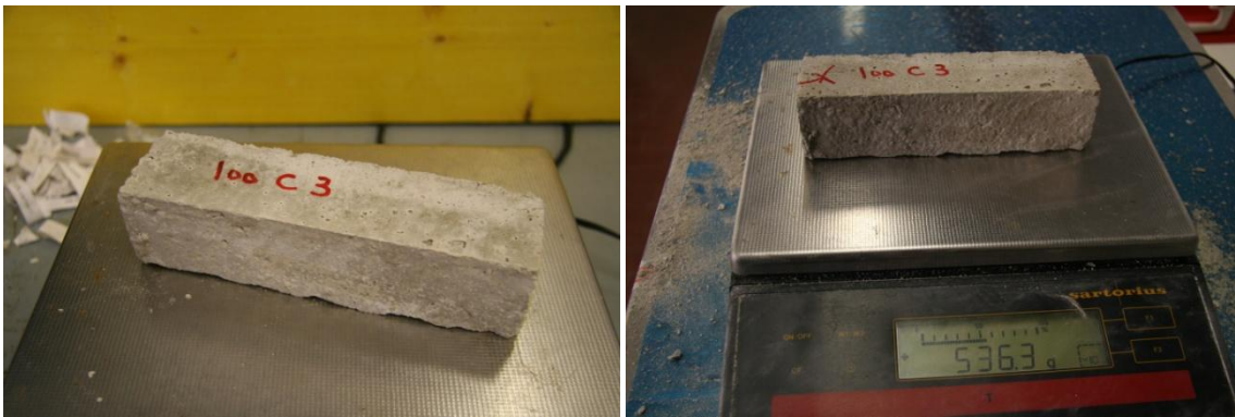
Fig 188 100% Cement Sample 3 Right after 93 Cycles, Left New sample
