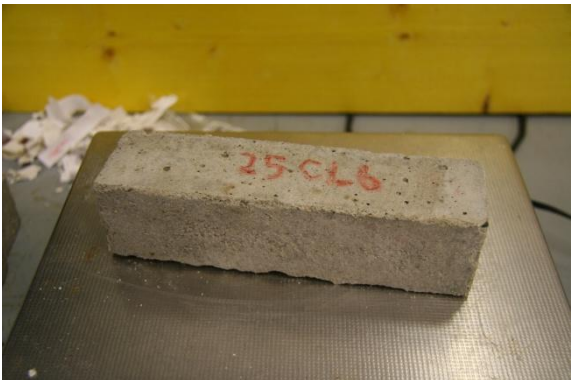
Fig 116 25% Cement Lime Sample 6 Right after 50 Cycles, New sample
