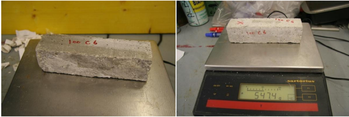
Fig 146 100% Cement Sample 6 Right after 50 Cycles, Left New sample
