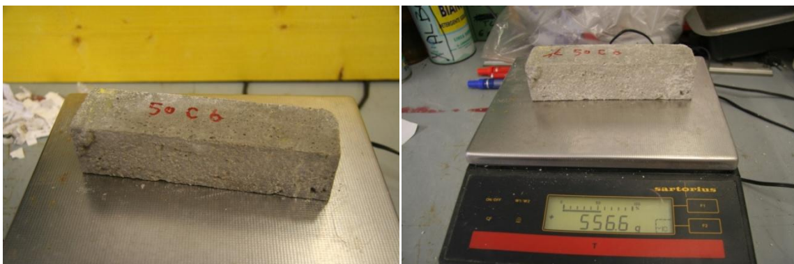
Fig 141 50% Cement Sample 6 Right after 50 Cycles, Left New sample
