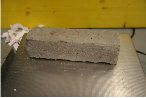
Fig 114 0% Cement Lime Sample 9 Right after 50 Cycles, New sample
