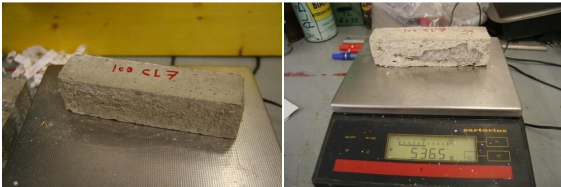
Fig 127 100% Cement Lime Sample 7 Right after 50 Cycles, Left New sample
