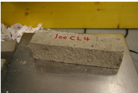
Fig 169 100% Lime Cement Sample 4 Right after 93 Cycles, Left New sample
