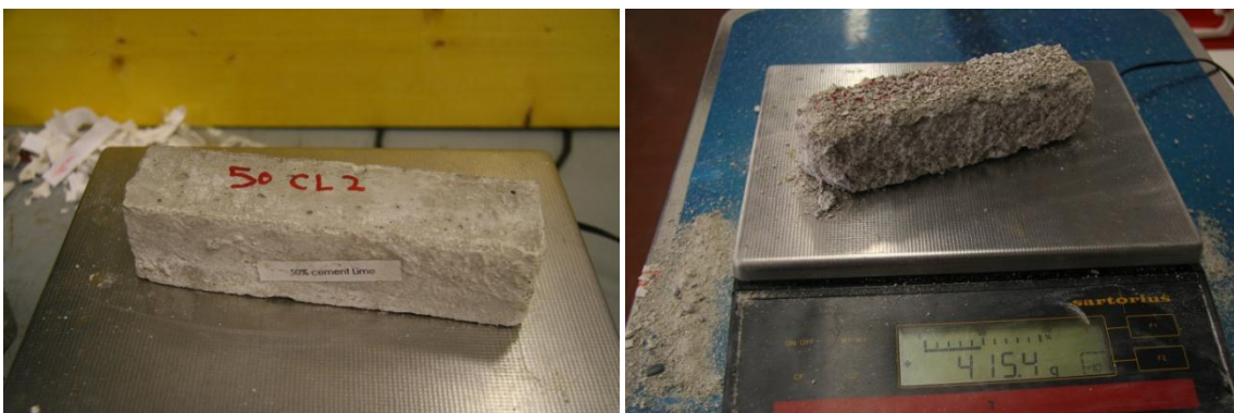
Fig 162 50% Lime Cement Sample 2 Right after 93 Cycles, Left New sample
