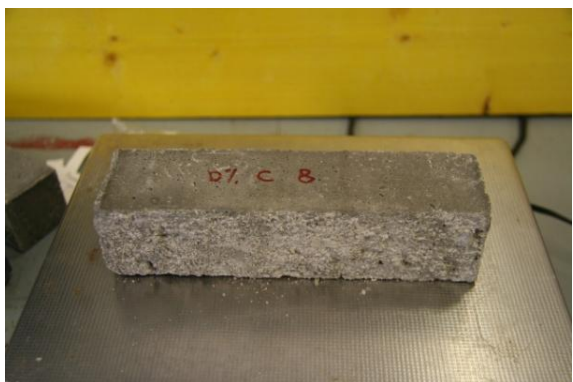
Fig 133 0% Cement Sample 8 Right after 50 Cycles, Left New sample
