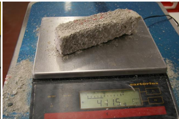
Fig 164 50% Lime Cement Sample 4 Right after 93 Cycles, Left New sample
