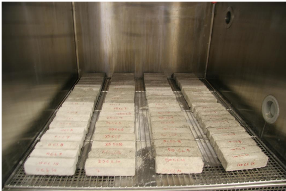
Fig 104 Degradation Test inside Chamber 30 th Oct
