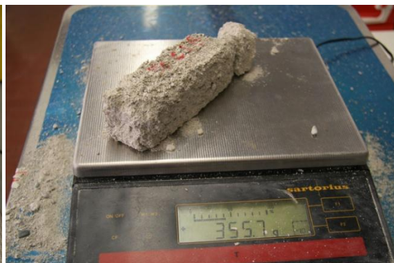
Fig 165 50% Lime Cement Sample 5 Right after 93 Cycles, Left New sample
