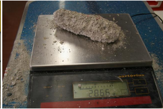
Fig 167 100% Lime Cement Sample 2 Right after 93 Cycles, Left New sample
