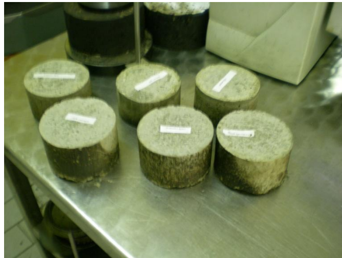
Fig 86 Samples for modulus of elasticity of mortar
