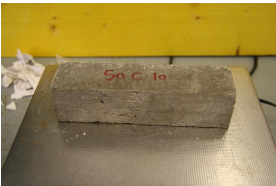
Fig 145 50% Cement Sample 10 Right after 50 Cycles, Left New sample
