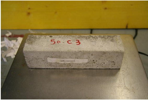
Fig 183 50% Cement Sample 3 Right after 93 Cycles, Left New sample
