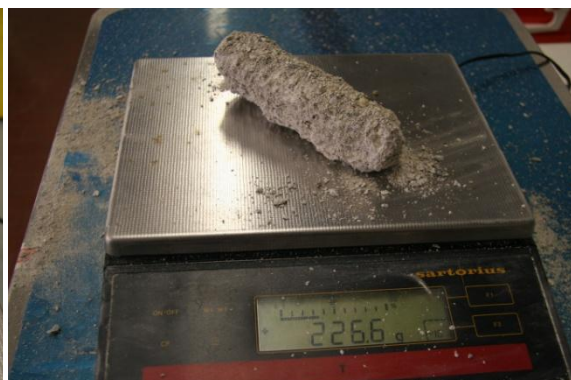
Fig 170 100% Lime Cement Sample 5 Right after 93 Cycles, Left New sample
