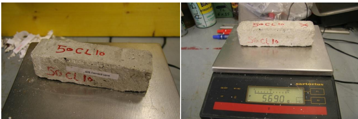
Fig 125 50% Cement Lime Sample 10 Right after 50 Cycles, Left New sample
