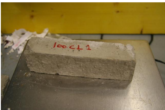
Fig 166 100% Lime Cement Sample 1 Right after 93 Cycles, Left New sample
