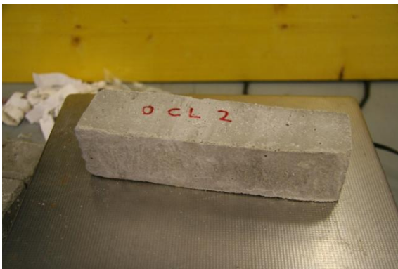
Fig 152 0% Lime Cement Sample 2 Right after 93 Cycles, Left New sample
