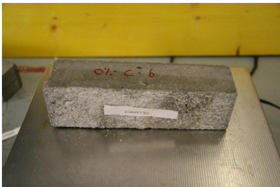
Fig 131 0% Cement Sample 6 Right after 50 Cycles, Left New sample
