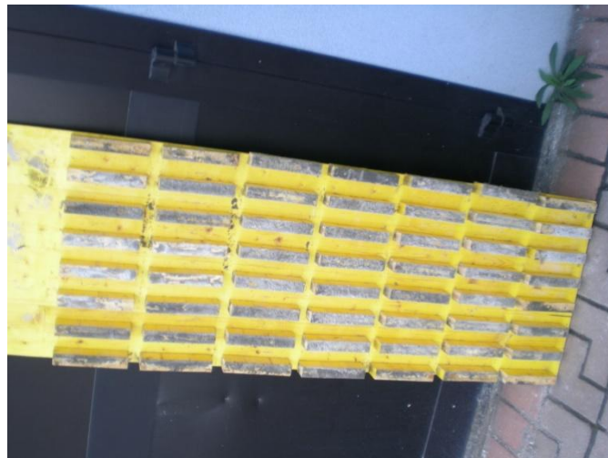
Fig 84 Mould made of wood to produce samples 16x4x4cm
