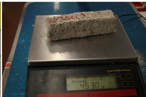
Fig 157 25% Lime Cement Sample 2 Right after 93 Cycles, Left New sample
