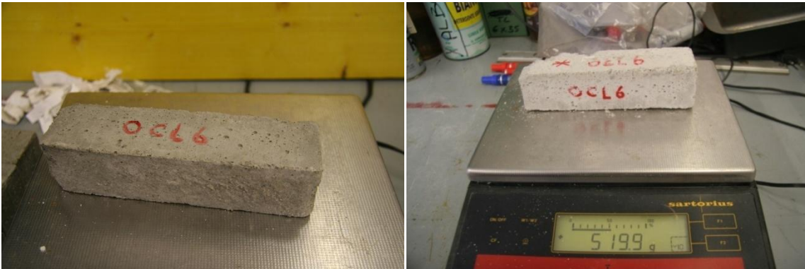
Fig 111 0% Cement Lime Sample 6 Right after 50 Cycles, New sample
