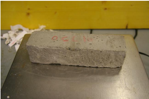
Fig 115 0% Cement Lime Sample 10 Right after 50 Cycles, New sample
