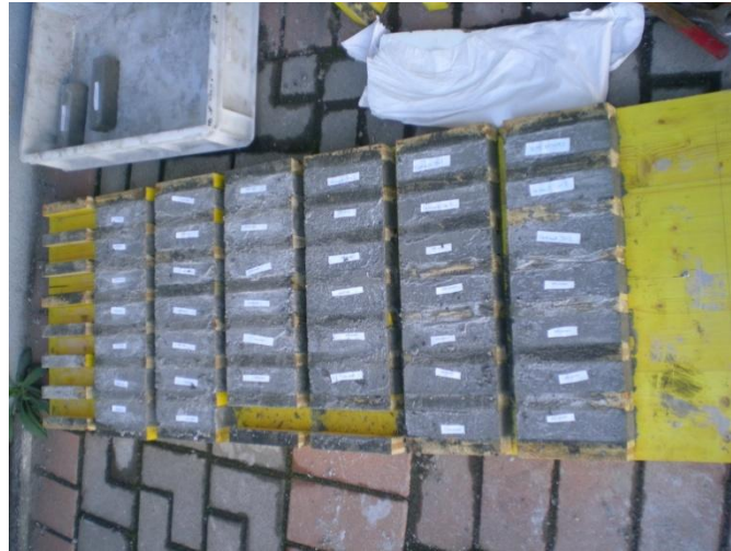
Fig 85 Mould made of wood to produce samples 16x4x4cm
