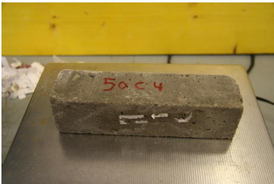
Fig 184 50% Cement Sample 4 Right after 93 Cycles, Left New sample
