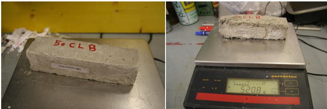
Fig 107 50% Cement Lime Sample 8 Right after 50 Cycles, Left New sample
