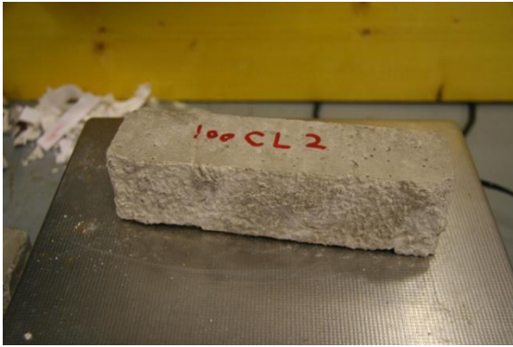
Fig 167 100% Lime Cement Sample 2 Right after 93 Cycles, Left New sample
