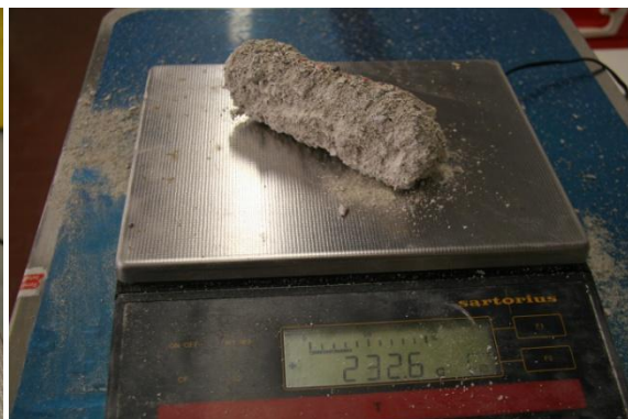
Fig 169 100% Lime Cement Sample 4 Right after 93 Cycles, Left New sample
