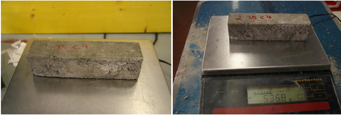
Fig 179 25% Cement Sample 4 Right after 93 Cycles, Left New sample
