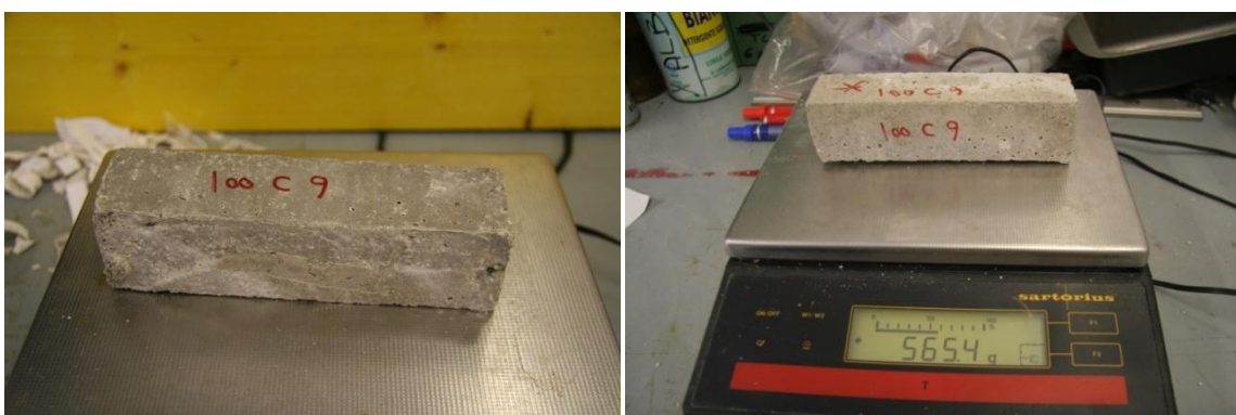
Fig 149 100% Cement Sample 9 Right after 50 Cycles, Left New sample
