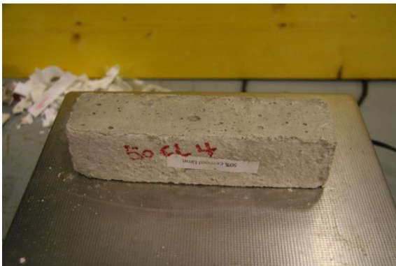
Fig 164 50% Lime Cement Sample 4 Right after 93 Cycles, Left New sample
