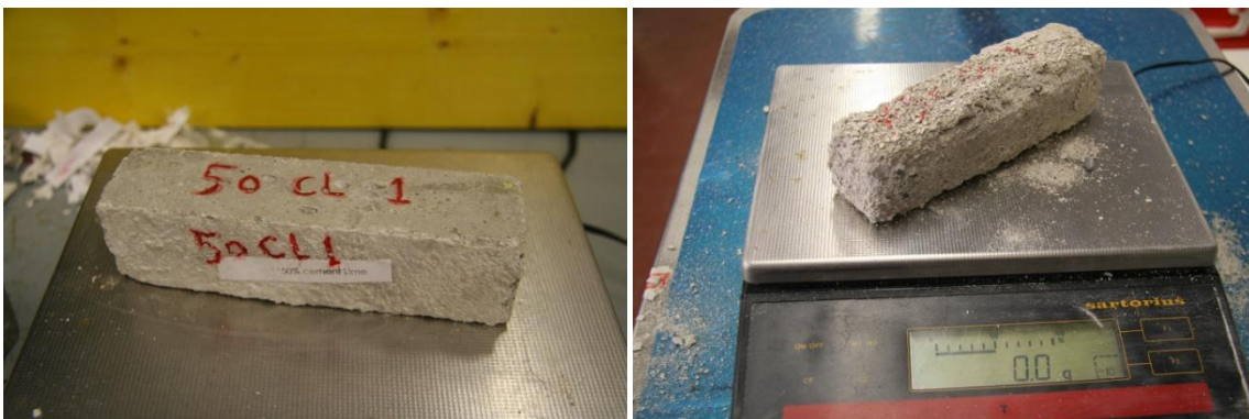
Fig 161 50% Lime Cement Sample 1 Right after 93 Cycles, Left New sample
