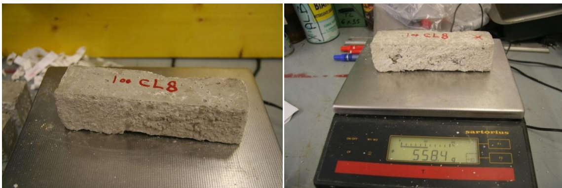
Fig 128 100% Cement Lime Sample 8 Right after 50 Cycles, New sample
