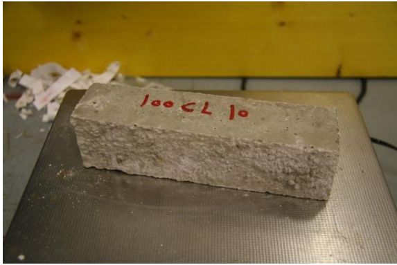
Fig 130 100% Cement Lime Sample 10 Right after 50 Cycles, Left New sample
