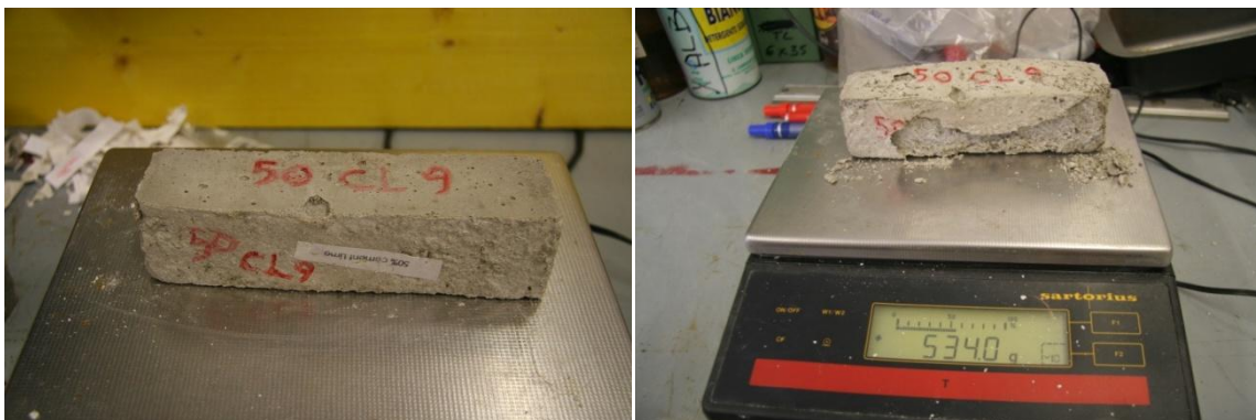
Fig 124 50% Cement Lime Sample 9 Right after 50 Cycles, Left New sample
