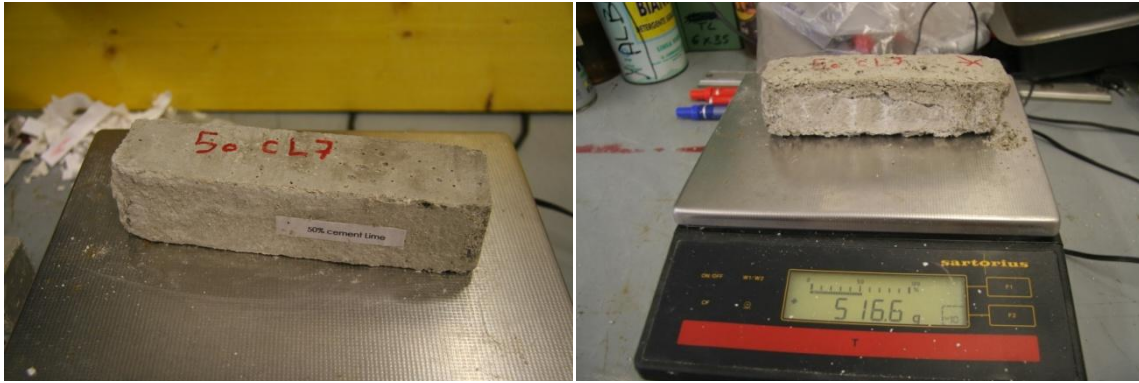
Fig 122 50% Cement Lime Sample 7 Right after 50 Cycles, Left New sample
