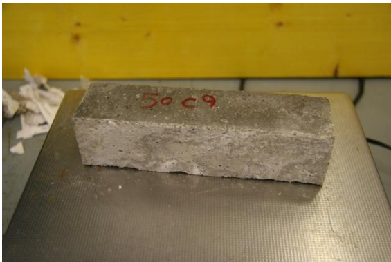
Fig 144 50% Cement Sample 9 Right after 50 Cycles, Left New sample
