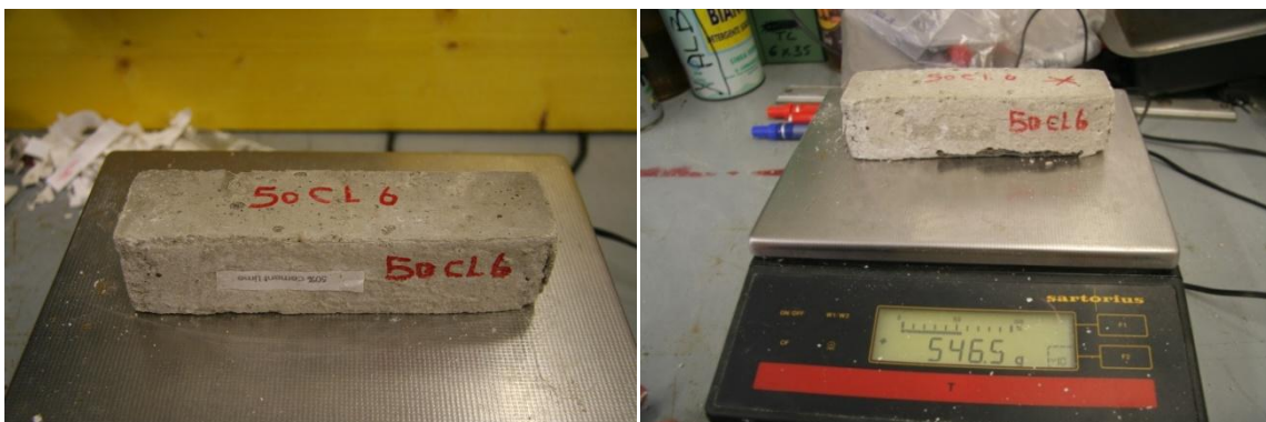
Fig 121 50% Cement Lime Sample 6 Right after 50 Cycles, Left New sample
