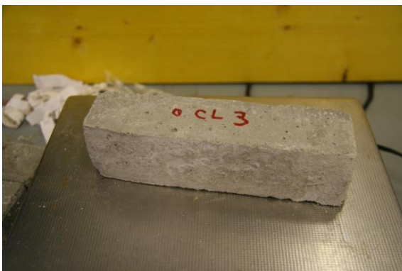
Fig 153 0% Lime Cement Sample 3 Right after 93 Cycles, Left New sample
