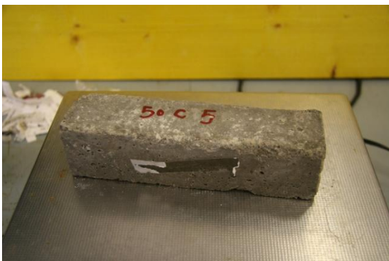
Fig 185 50% Cement Sample 5 Right after 93 Cycles, Left New sample
