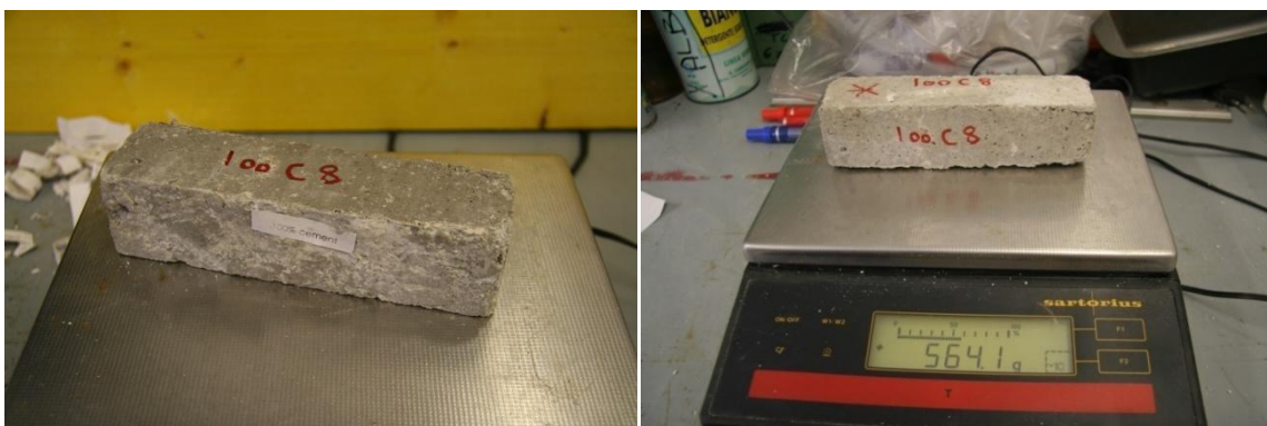
Fig 148 100% Cement Sample 8 Right after 50 Cycles, Left New sample
