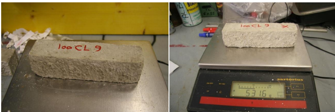
Fig 129 100% Cement Lime Sample 9 Right after 50 Cycles, Left New sample
