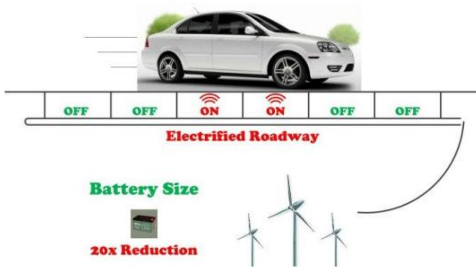
Figure1.3: Electrified roadway concept.
