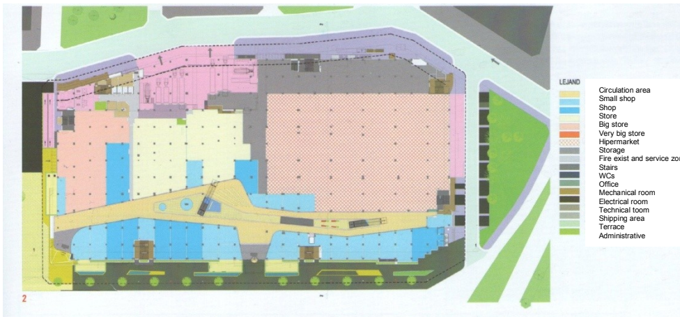
Fig. 6-24: Ground floor plan
