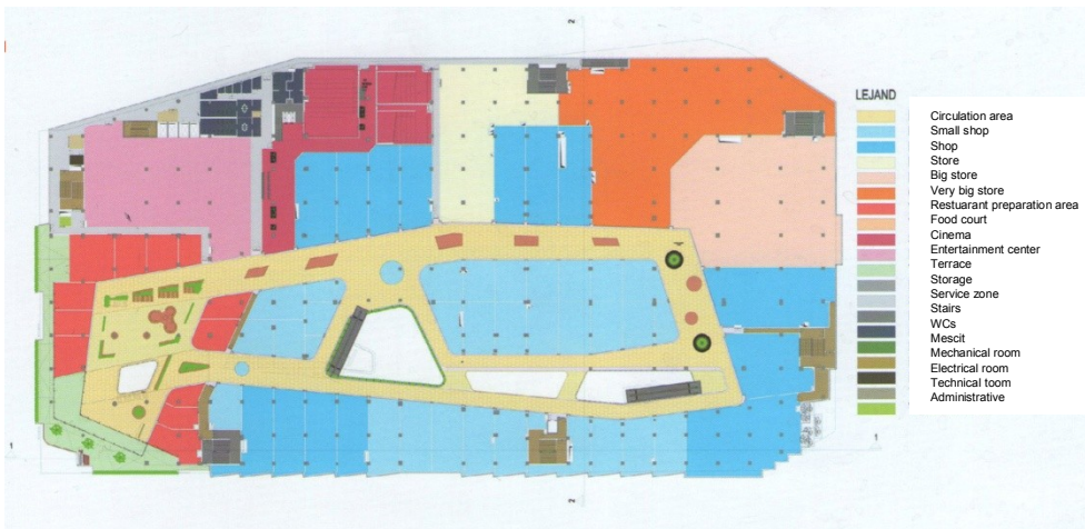
Fig. 6-25: First floor plan
