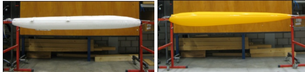
FIG. 3.4-5: MOCK-UPS TO STUDY THE FORM FINDING OF INFLATABLE TENSAIRITY ® HULLS
