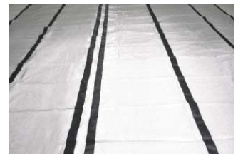
FIG. 3.55: TARPAULIN WITH REINFORCED BANDS
