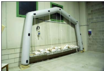
FIG. 4.74: TEST OF PROTOTYPE 4 WITH A LOAD BEARING CAPACITY 2 TIMES HIGHER
