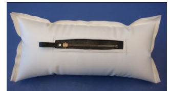
FIG. 4.77: AIR TIGHTNESS TESTS ON A ZIP
