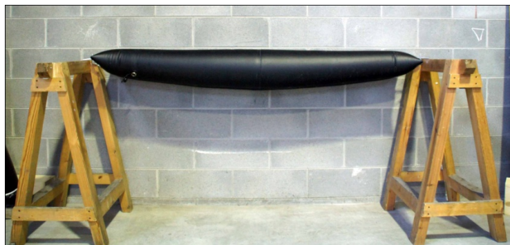
FIG. 4.24-25: LINEAR BEAMS: STANDARD "O SECTION" (GREY) AND TENSAIRITY ® WEB VERSION (BLACK)
