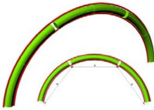
FIG. 3.56: STUDY ABOUT DIVISION OF THE INFLATABLE ARCH INTO SHORTER SEGMENTS
