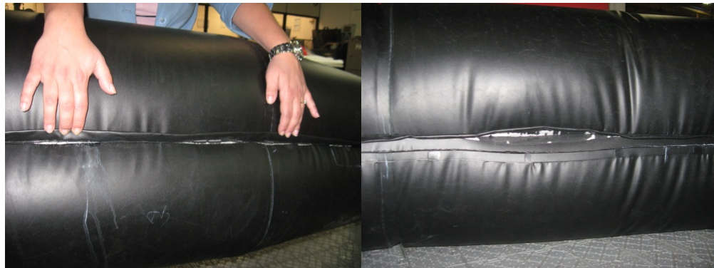
FIG. 4.45-46: DAMAGES DUE TO PEELING AFTER ONLY ONE DAY OF INFLATION
