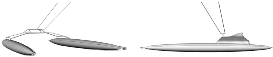
FIG. 4.17-18: FIRST DESIGN OF THE INFLATED CATAMARAN
