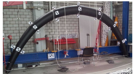
FIG. 4.41-42-43: SMOOTH TENSAIRITY® ARCH: DESIGN, DIMENSIONS AND PROTOTYPE
