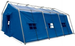
FIG. 3.12: FAST SET UP 6X6 W/L/H: 5,9/5,9/28 M AREA: 34,6 M2 WEIGHT: 327 KG KG/M 2 = 9,4
