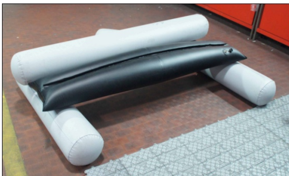
FIG. 4.24-25: LINEAR BEAMS: STANDARD "O SECTION" (GREY) AND TENSAIRITY ® WEB VERSION (BLACK)
