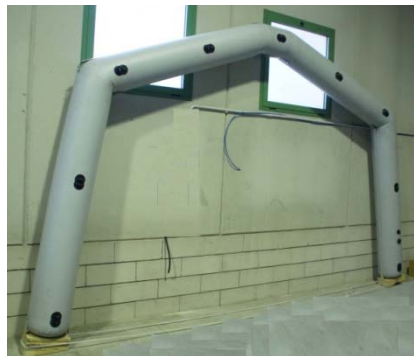
FIG. 4.34-35: TENSAIRITY SEGMENTED ARCH: DESIGN AND PROTOTYPE
