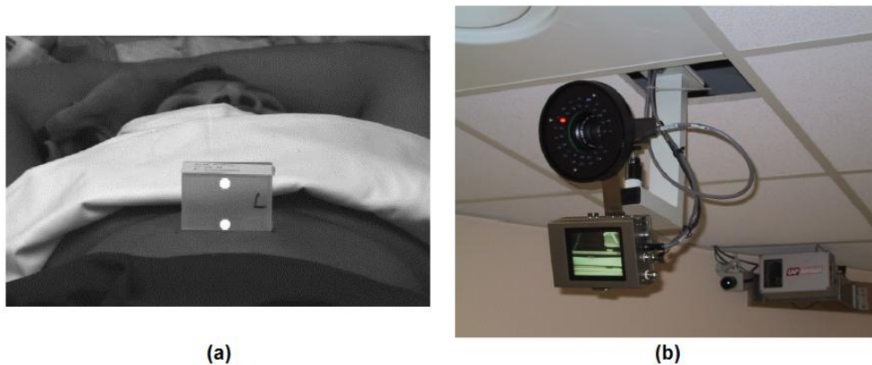
Figure 1.15. RPM optical system for the tracking of external surface motion. The device is composed by a plastic block with passive reflective markers placed on the patient's abdomen (Panel a). The AP trajectory of the block is recorded by a ceiling-mounted CCD camera, equipped with infrared light-emitting diodes for marker illumination (Panel b).
