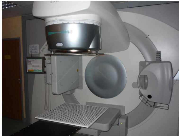
Figure 3.6. Photo of the planar grid of black spots used for the calibration of the VisionRT surface imaging system.
