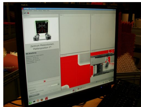
Figure 3.26: ARAMIS camera calibration
