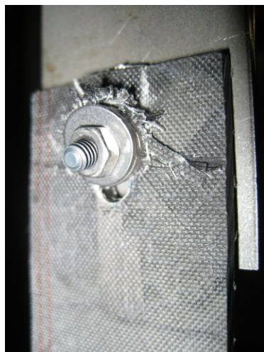
Figure 6.17: Configuration 2, coupon 7, bearing deformation
