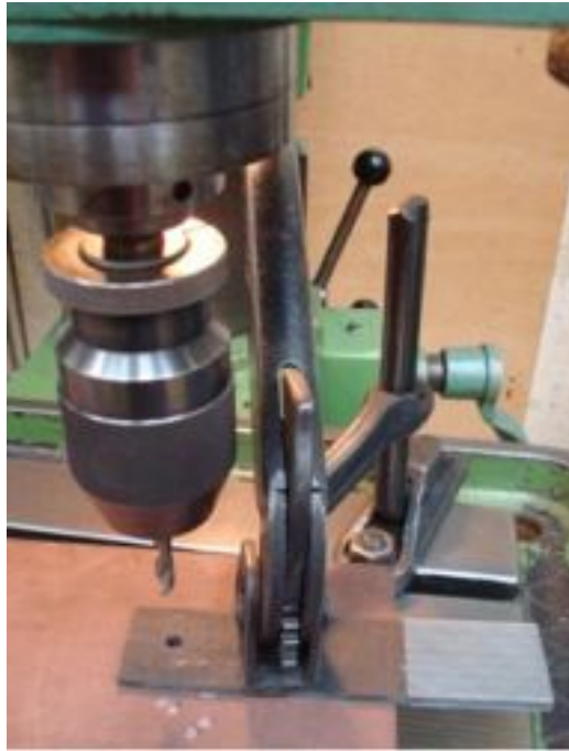
Figure 3.21: Drilling on a bearing coupon
