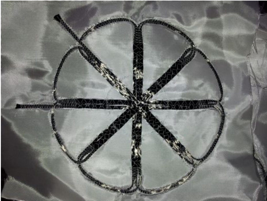
Figure 3.5: Single star patch with 3 roving not refined
