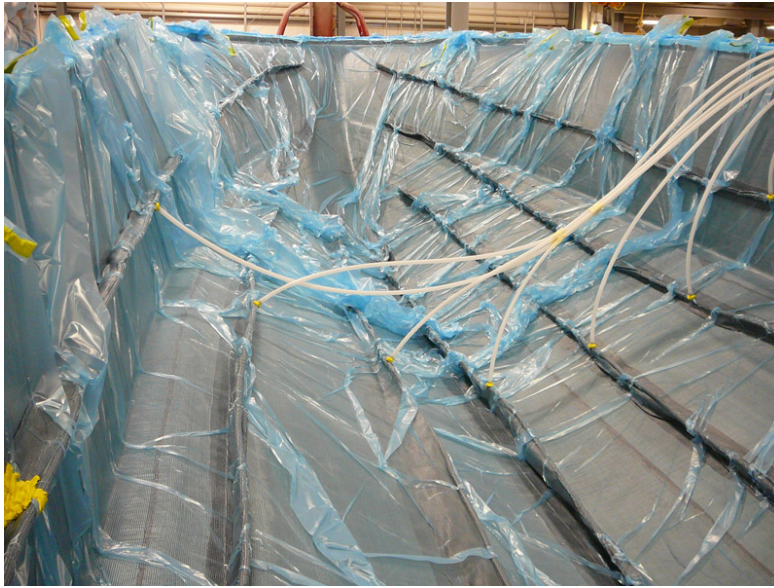
Figure 2.7: Vacuum Infusion Technology: Hull, Southport boat [8]
