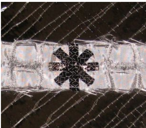
Figure 3.6: Star patches reinforcements, 3 rovings per arm
