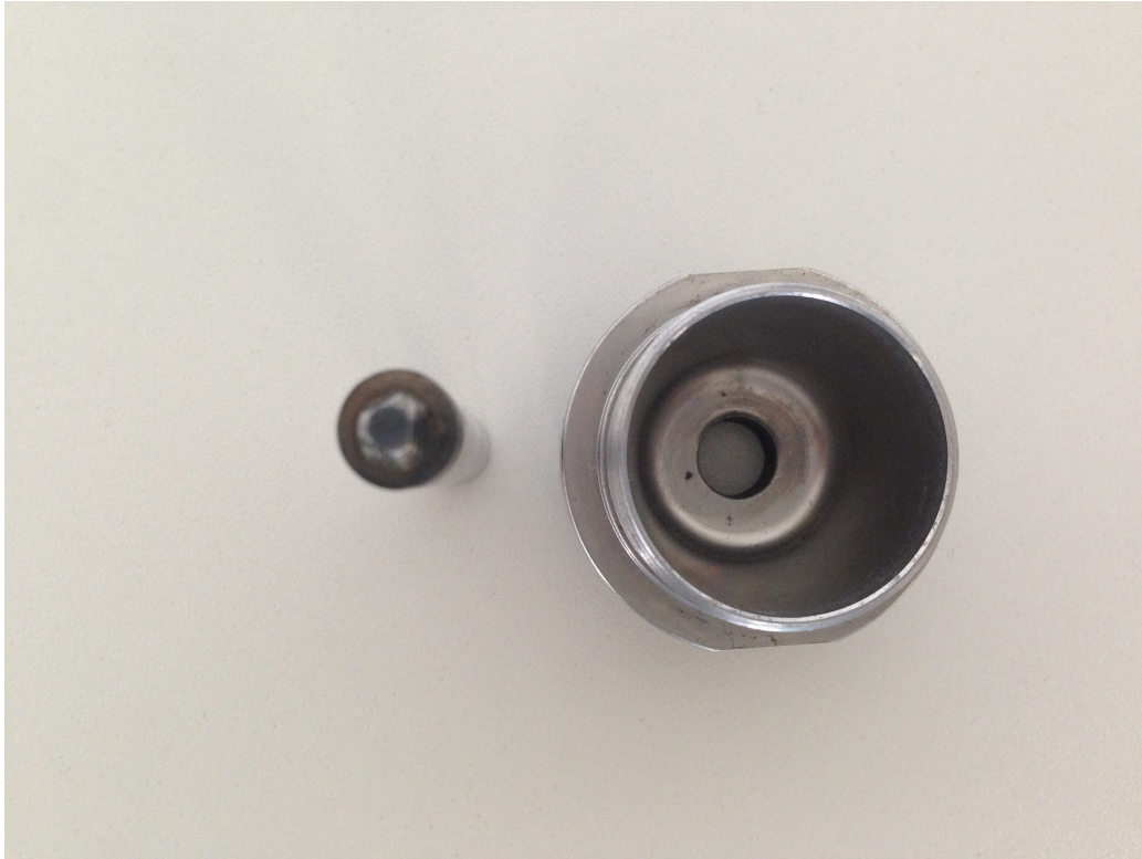
Figure 3.18: Effect of forces applied during FSW on an unhardened shoulder and pin used during testing
