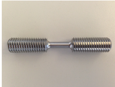
Figure 2.28: Particular of screws with a reduced midlength cross section
