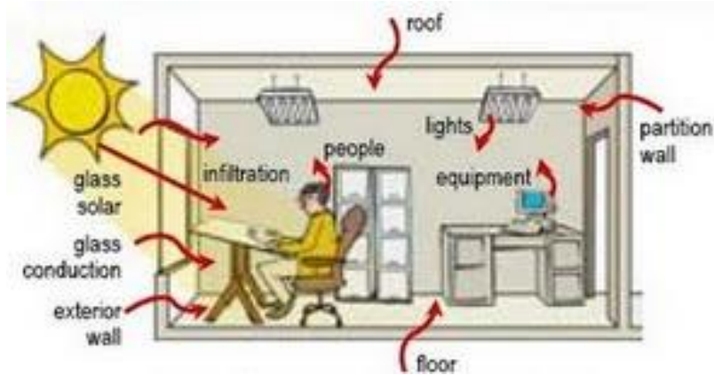
Fig. 5.16: Different means of heat gain in a living space. 7
