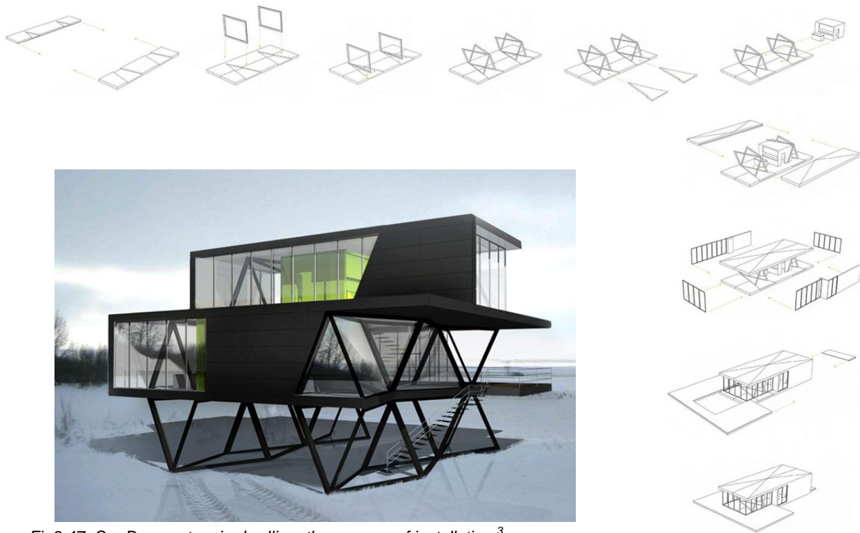
Fig3.47: QuaDror system in dwelling, the process of installation 3
