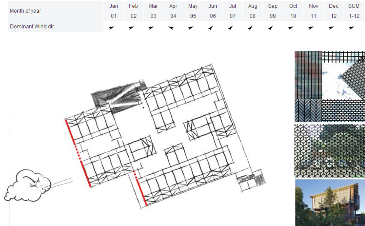
Fig. 5.23: A scheme showing the sheltered area from the prevailing wind. 10
