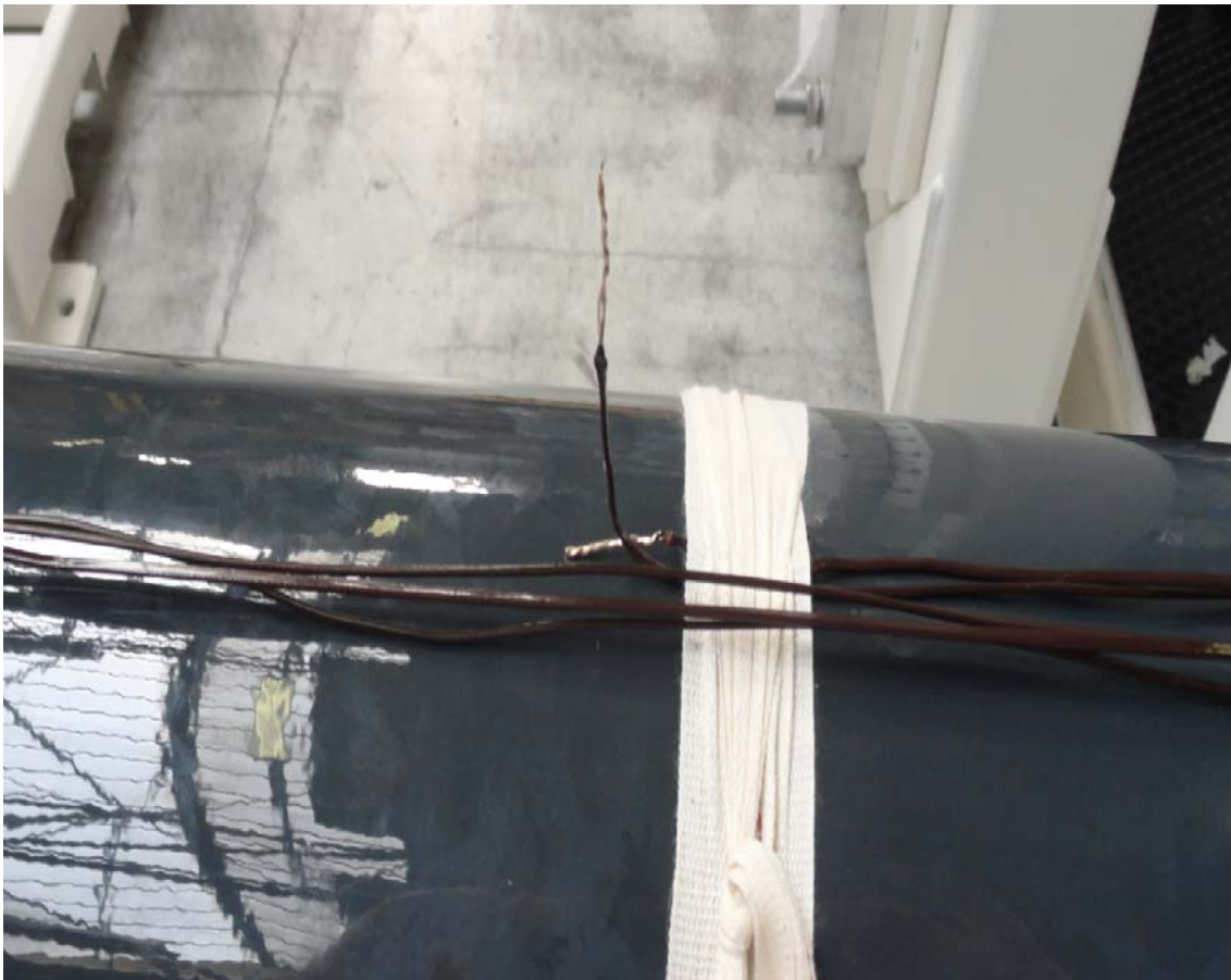
Figure 2.2 - Two Thermocouples Positioned on the Conductor of the PHI Bushing, in the Gas Side: One is Placed Along the Conductor to Measure its Temperature in That Zone, One is Up in Air to Measure the Internal Gas Temperature.
