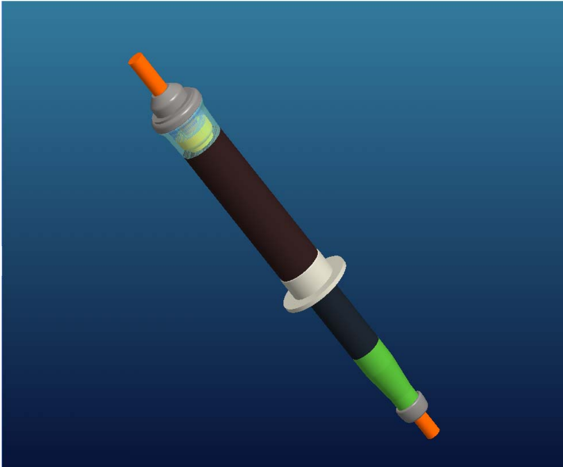
Figure 4.1 - Mechanical Bushing Model in Order to Realize a Thermal Simulation
