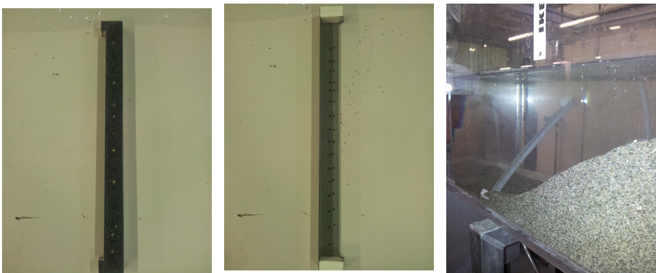
Fig.2.31. Object for calibration the laser (From left to right: Rough surface, smooth surface, position n the channel)
