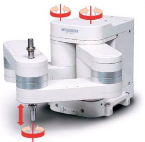
Figura 2.1: Robot pentalatero Mitsubishi RP.
