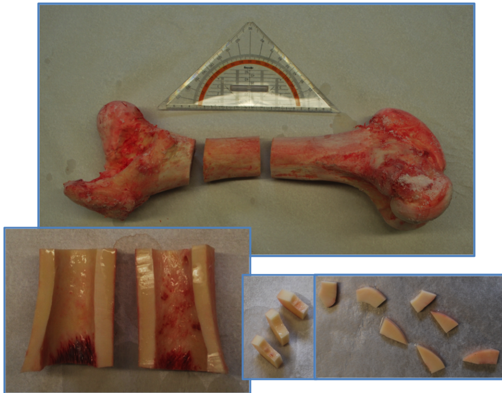
Figure 2.6: Bovine bone specimens preparation.
