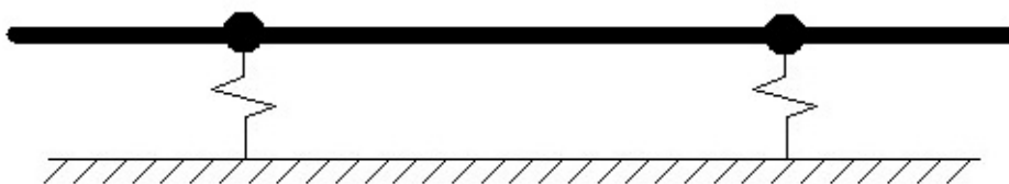
Figure 3.1: Scheme of the FE model of the track
