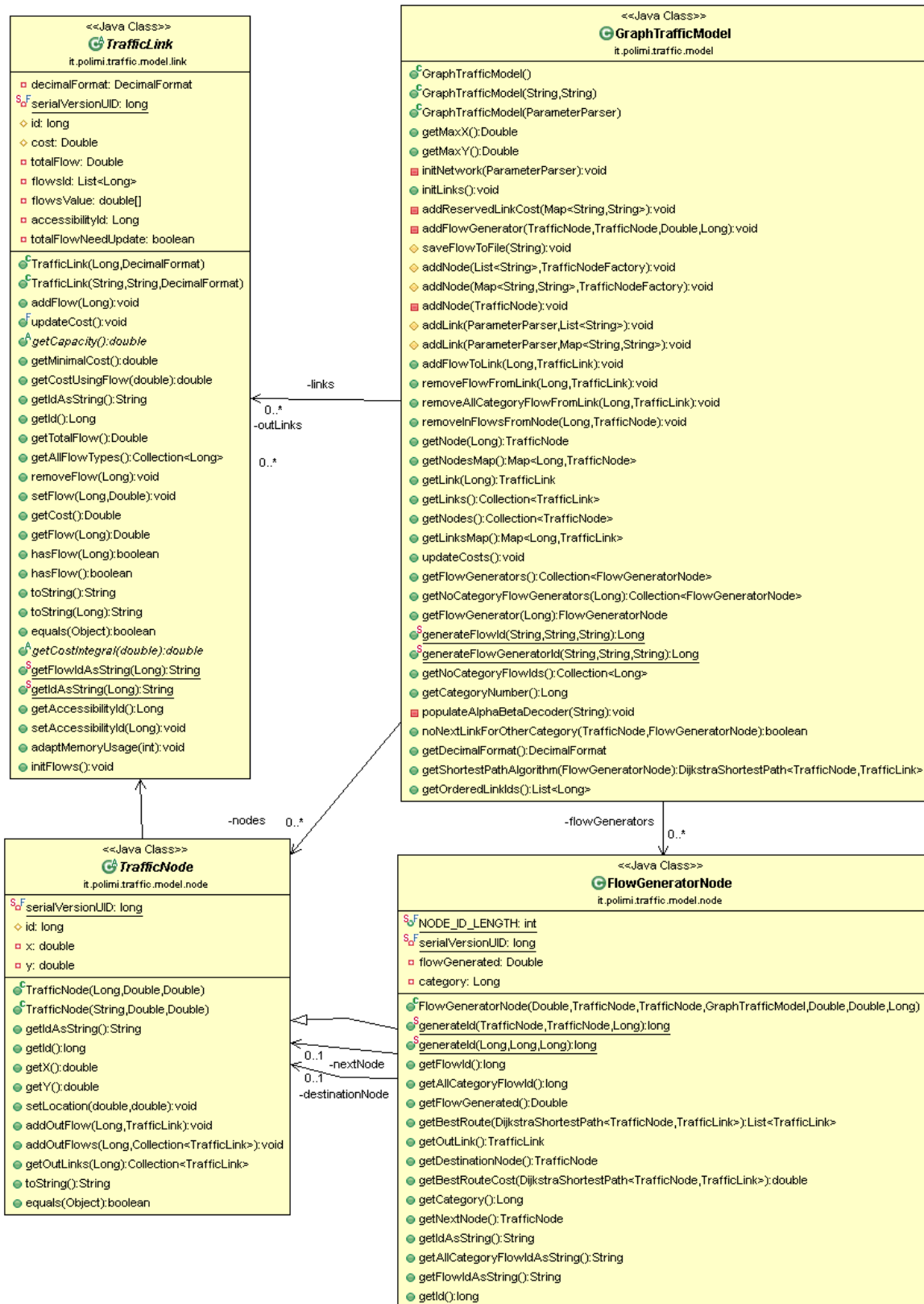
Fig. 4.1: Class diagram for the network model
