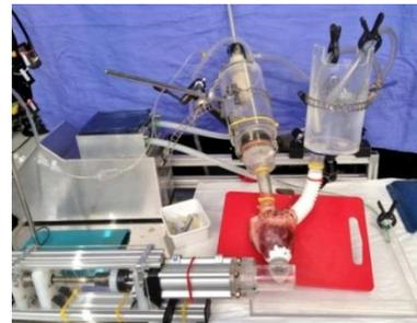
**Figure 1** Pulsatile mock loop for entire porcine explanted hearts developed by Leopaldi *et al.* [1].
