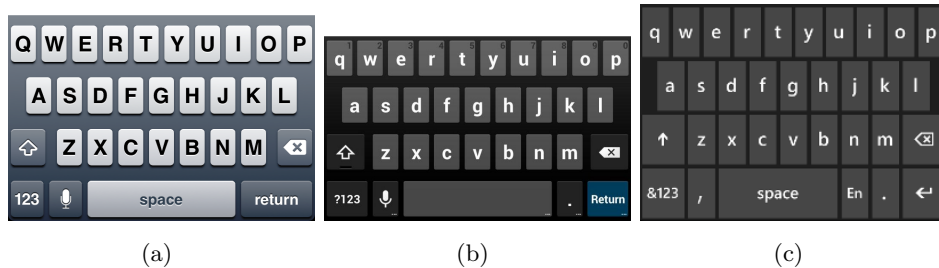
Figure 2.2: The QWERTY soft keyboards of (a) iPhone, (b) Android, (c) Windows Phone
