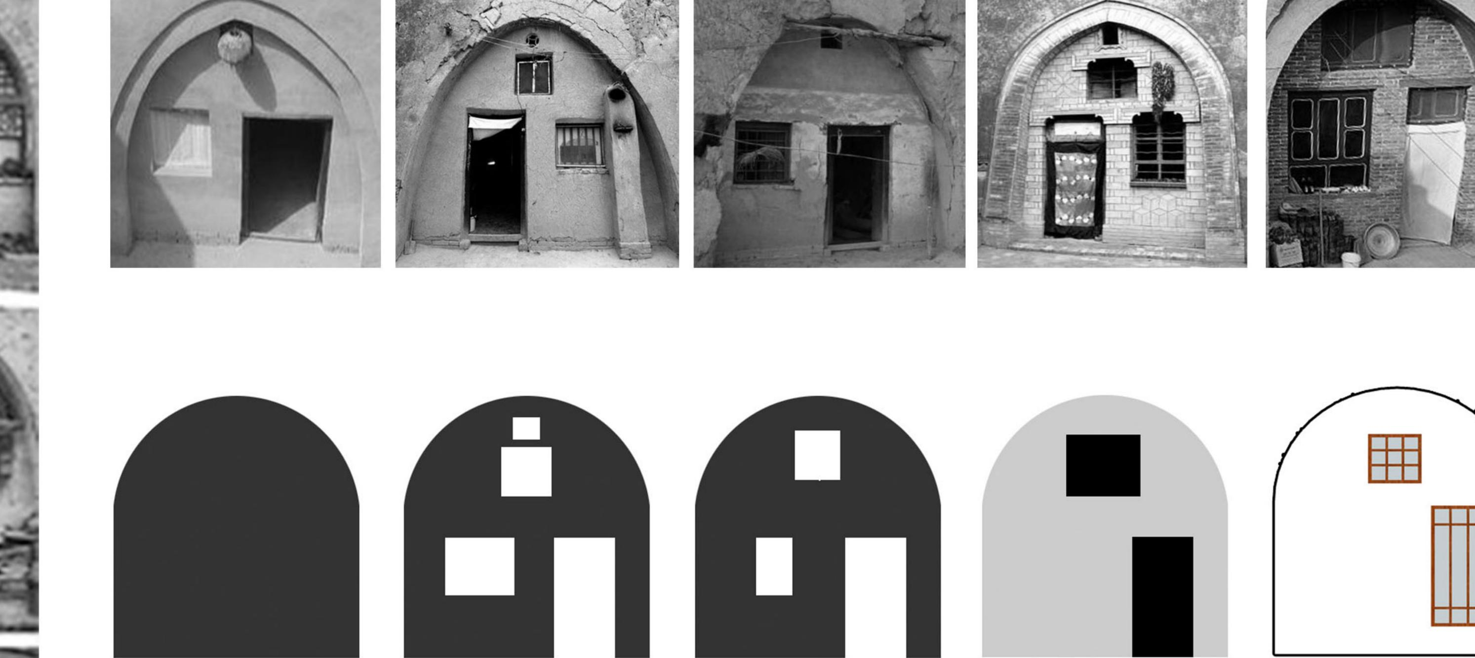
The two different types of "face" are the initial concept to design the new façade of Yaodong caves. In the hope of preserving the identity of Yaodong building, the position of substance and void remains almost the same. However, constructed with new insulation materials, the physical character for this façade is highly improved.
