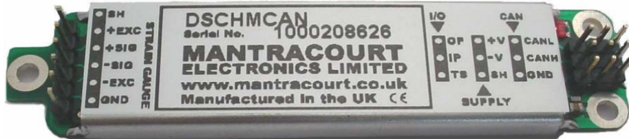
Figure 2.14: Mantracourt DSC Load Cell Embedded Digitiser
