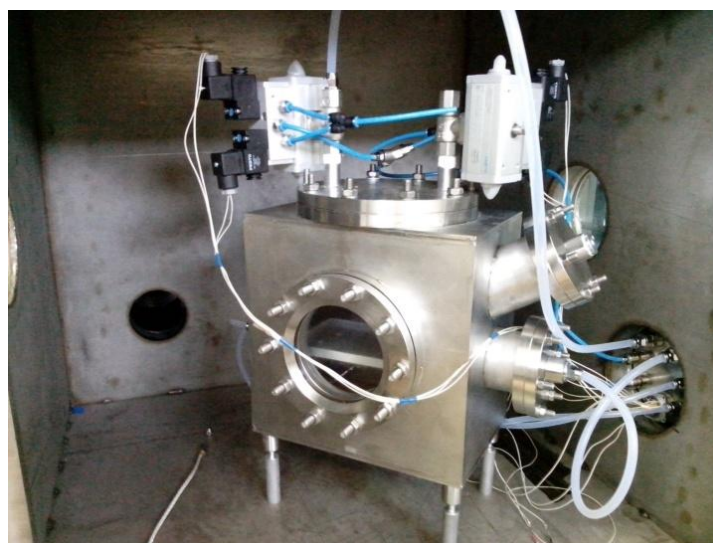
Fig. 74: Experimental installation's Injectors
