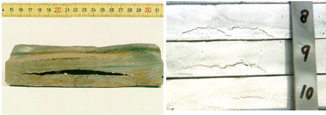
Figure 1.2 - On the left, example of blistering; on the right, SWC typical form [2].
