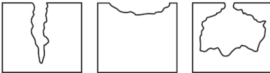
Figure 1.2- Typical shape of pitting corrosion attack [4].
