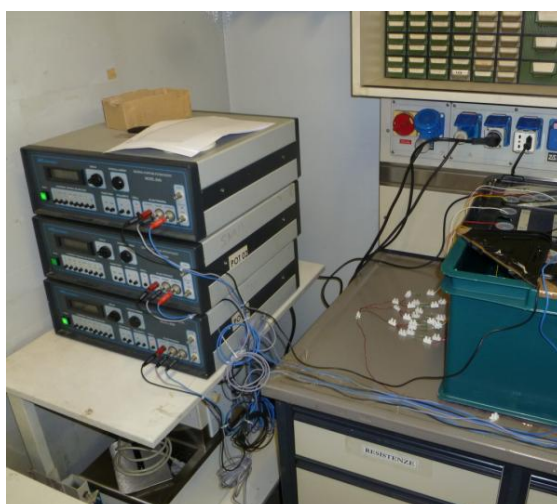
Fig. 3.9- Electrical connection of the electrochemical cells to the potentiostat.
