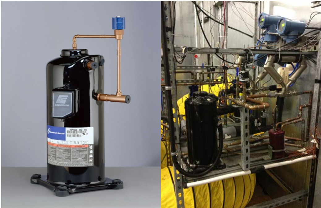
Figure 2.1. Picture of a digital scroll compressor (left) and picture of a digital scroll compressor mounted in the experimental set-up (right).
