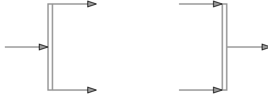
Figure 4.6: Parallel opening and closure
