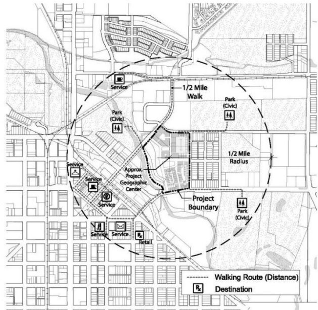
Figure 55 Walking routes on pedestrian network showing distances from dwellings and nonresidential uses to diverse use destinations
