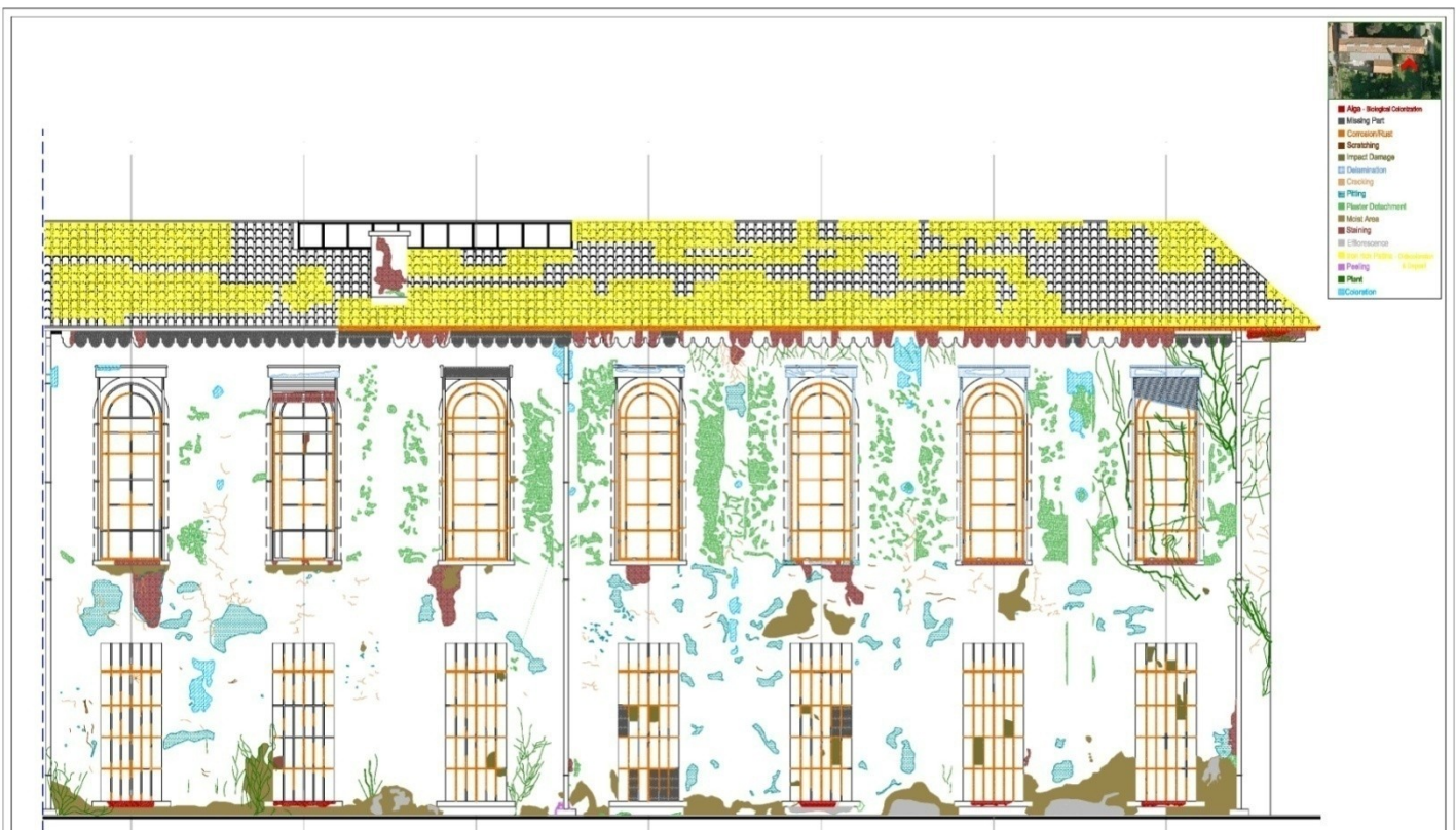
Figure 39 Sample of the facade material survey
