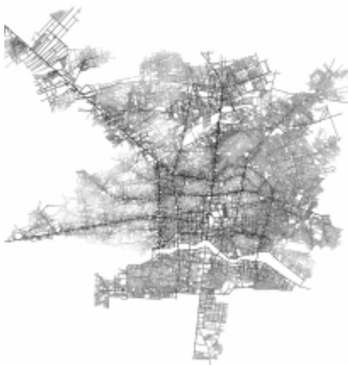
Axial analysis of existing Isfahan (2002), showing the measures of spatial integration (global integration). The darkest line on the map has the most and the lightest line has the least integration value.
