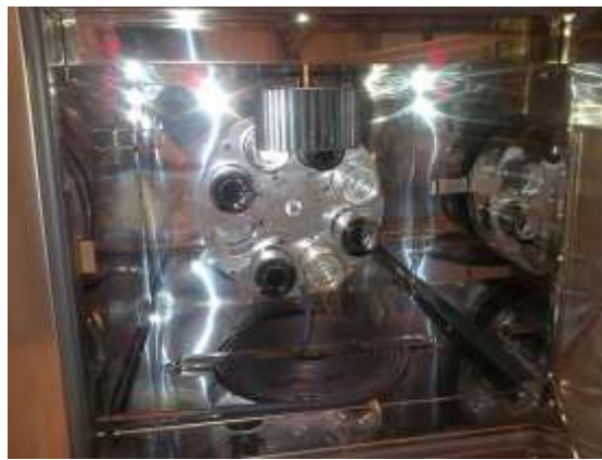
Figura 3.2-11: Stufa a tamburo rotante (Rolling Thin Film Oven)
