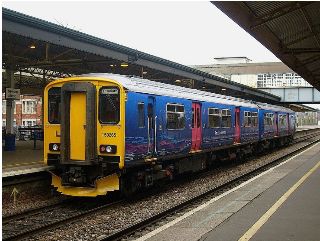
Figure 2.45: Photo of the Class 150 Sprinter diesel multiple unit train. Reproduced from http://en.wikipedia.org/
