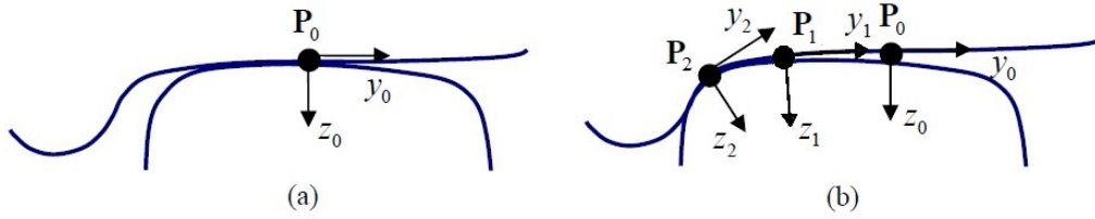
Figure 7.1: Typical wheel/rail contact position: (a) nominal contact position P_0 , (b) flange ( P_2 ) and tread ( P_1 ) contact positions during left curve negotiation
