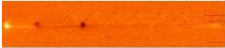
Figure 3.9: MFM image of a zig-zag magnetic conduit: dark and bright spots represent respectively an attractive or repulsive magnetic force, acting on the ferromagnetic tip.
