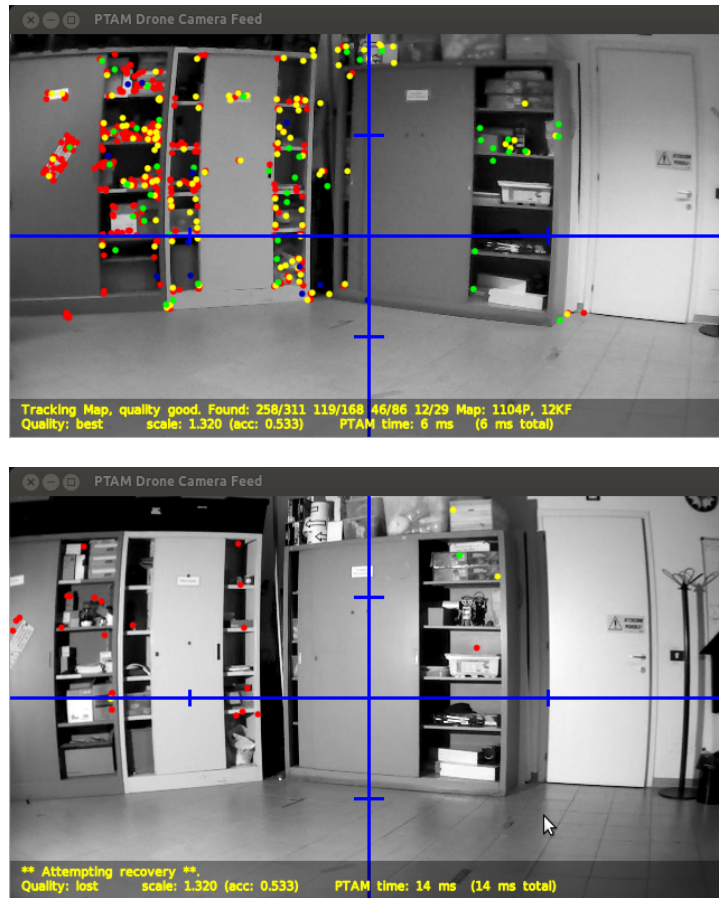
Figure 5.17: Effect of a sudden variation of light intensity in PTAM system.
