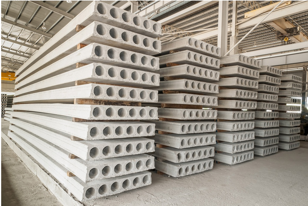
Figure 16: Reinforced precast concrete slabs
