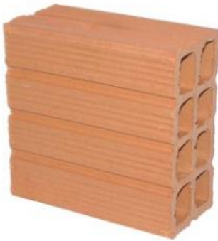
Figure 26: Traditional brick with holes, called in portuguese "tijolo baiano"
