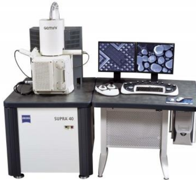
Figure 2.5 Zeiss® Supra 40 field emission scanning electron microscope (FE-SEM)
