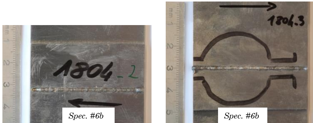
Figure 8.10: Macro-view (top and bottom in left and right pictures respectively) of laser welded surfaces using the #6b experimental condition
