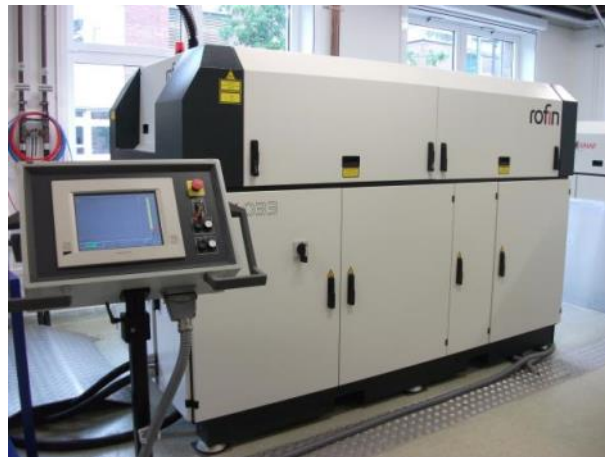
Figure 6.1: Rofin Sinar DY033 Nd:YAG laser source with control panel
