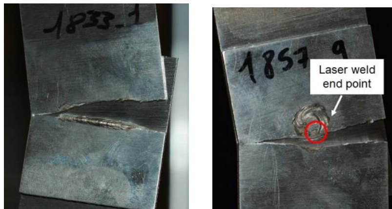
Figure 8.29: Cracks propagation in linear and circular laser welds
