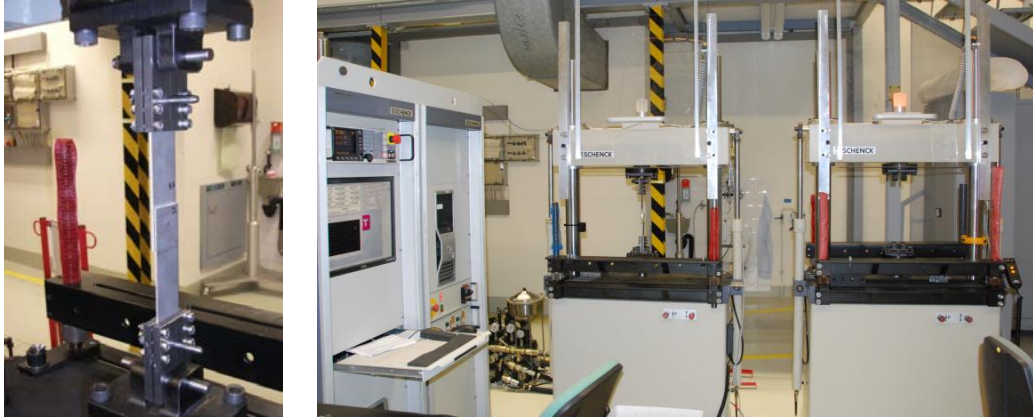
Figure 6.8: A running fatigue test and the full fatigue testing equipment
