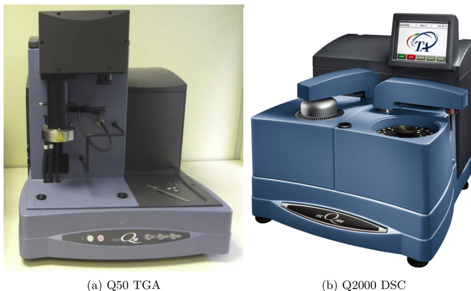
Figure 5.1: Photograph of the thermal analysis instrumentation used during this study, made by T.A. Instruments, inc.
