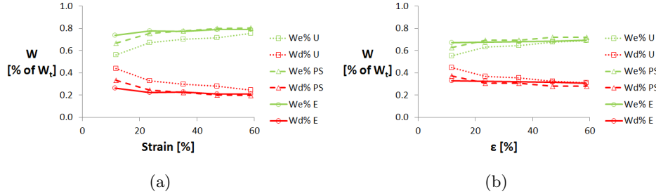
Figure 5.14: Elastically stored energy density W_e and dissipated energy density W_d as a percentage of W_t for different strain levels and loading conditions. a)NR and IR b)SBR.
