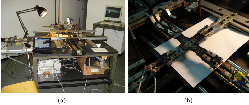
Figure 2.1: a) LaBS biaxial tester used for fracture test on cross shaped specimens; b) Cross shaped specimen mounted on the LaBS biaxial tester.
