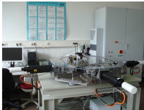
Figure 2.2: The Coesfeld Materialtest biaxial tester used for dynamic characterization and fatigue test.
