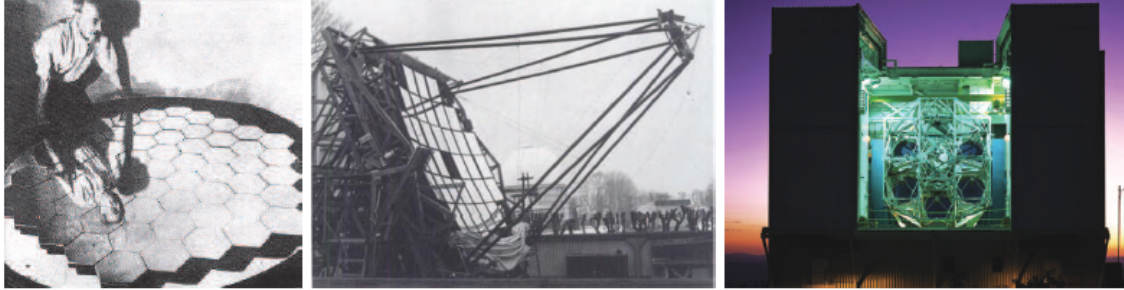
Figura 1.4: The first three segmented telescopes: the mirror of Horn d'Arturo, the segmented telescope of Pierre Connes and the MMT [37].
