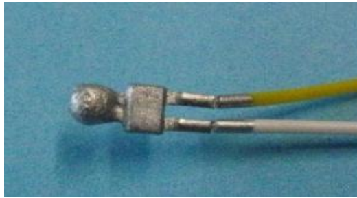
Figure 29: Electric igniter pill
