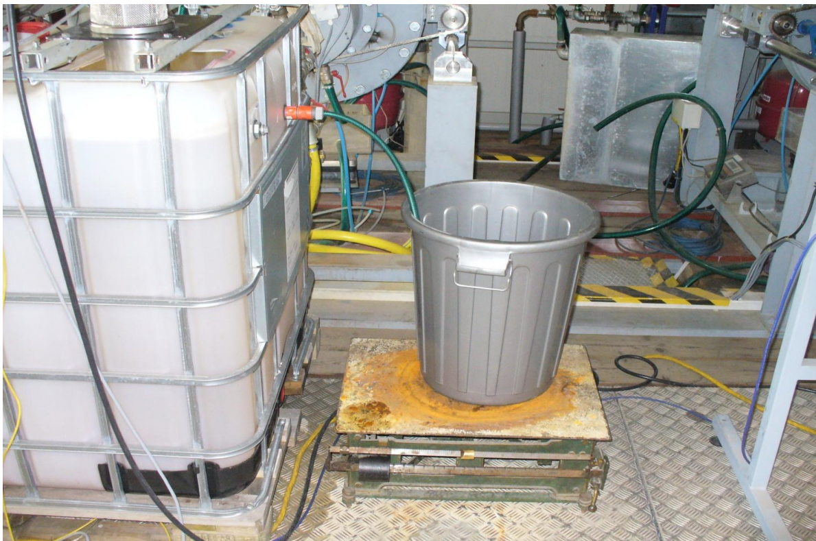
Figure 34: Test-rig for the measurement of leakage losses.
