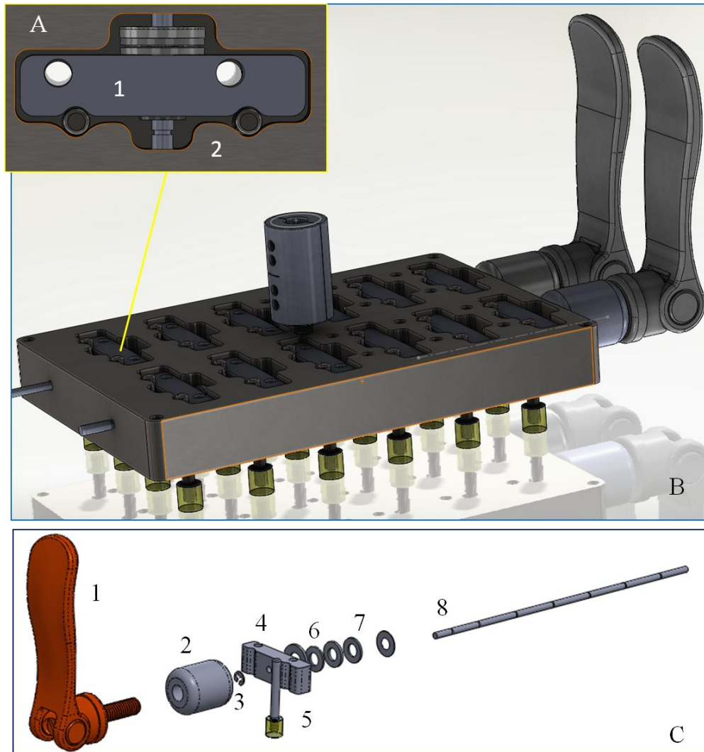
Figure 2.12. SolidWorks® representation of the clamping system. (A) Zoomed top view of two plungers clamped between the moving part (A1) and the fixed part (A2). (B) Trimetric view of the bioreactor's lid. (C) Exploded view of all the pieces composing the clamping system: 1) cam-lever, 2) standoff, 3) threaded nut, 4) moving part, 5) plunger, 6) Belleville spring, 7) Belleville washer, 8) threaded rod.
