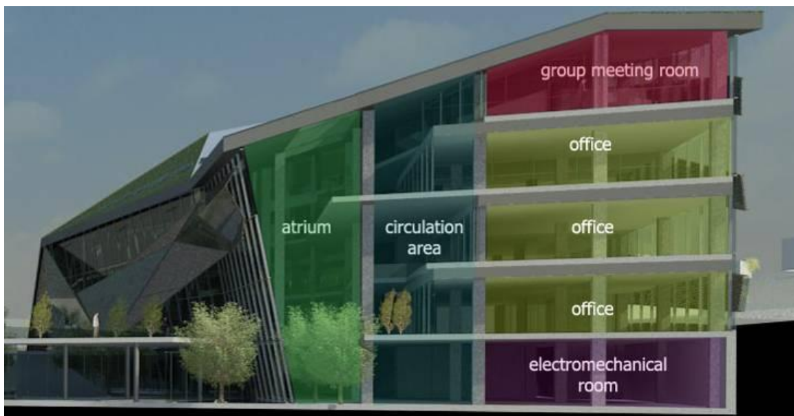
Figure 4.30 – Partial Section of the Building
