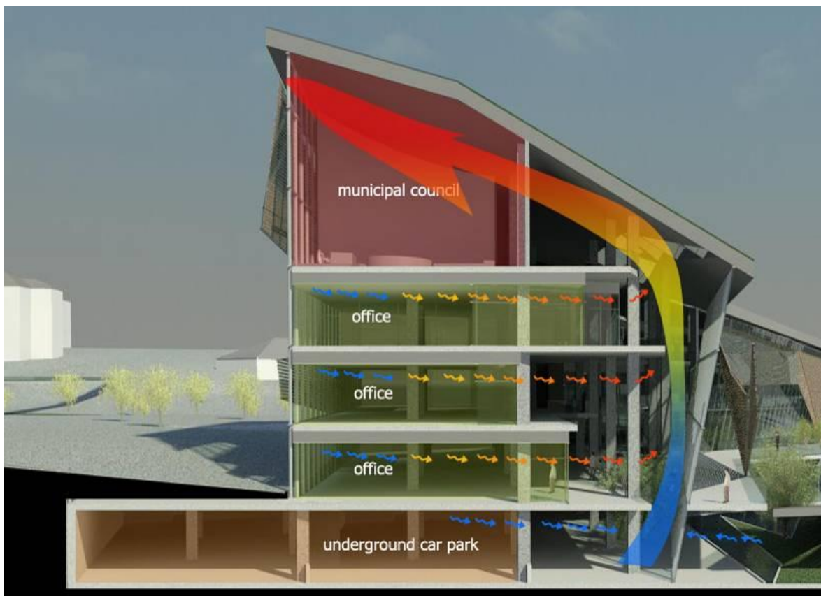
Figure 4.31 – Natural Ventilation Scheme
