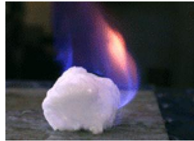
Figure 3.30- Hydrate on fire. Source: dco.gl.ciw.edu
