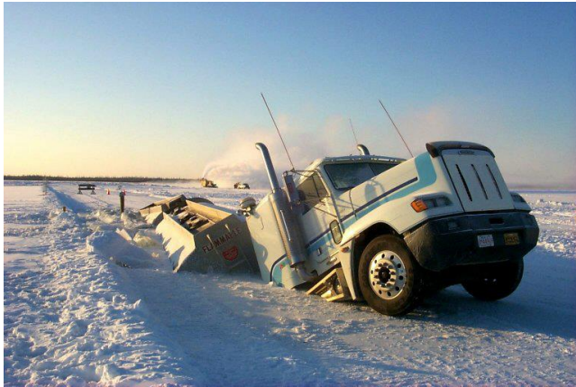
Figure 3.10-The danger of thin ice. A Super-B-Truck truck hauling diesel fuel broke through the Mackenzie River ice crossing near Fort Providence, Northwest Territories, Canada. Source: CBC news
