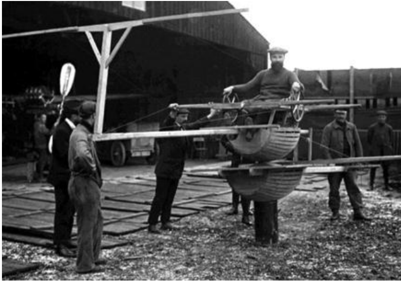
Figure 1.1. The "Antoniette Learning Barrel" simulator, 1910
