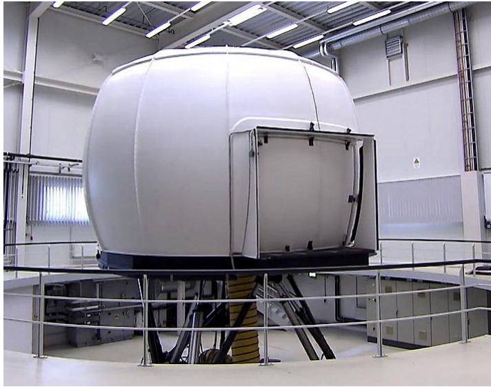
Figure 1.3. The BMW 6DOF simulator, 2003
