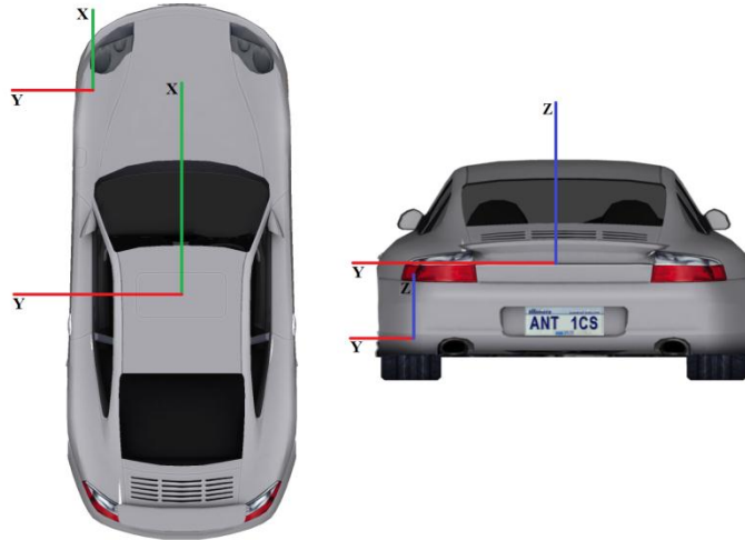
Figure 2.15. Speed Dreams' vehicle frame of reference
