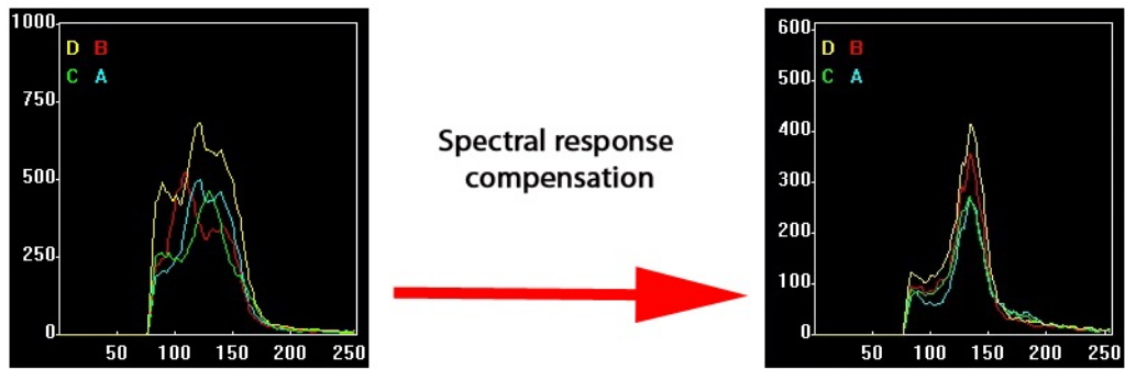
Figure 3.5: The spectral response for four neighboring PMTs (A-B-C-D), before (on the left) and after (on the right) correction
