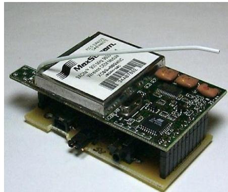
Fig. 2.8: RF and interface board [11].
