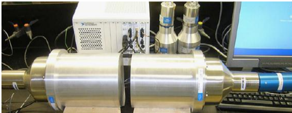
Fig. 2.3: Full system with NaI(Tl) detectors, PMTs and power supply [1].
