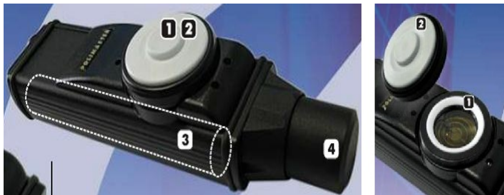
Fig. 2.2: Combined block to measure DER of photon radiations and both alpha and beta flux densities (1); Photon filter which ensures measurements of DER Hp(10); Neutron radiation detector (3); Gamma radiation detector (4) [3].
